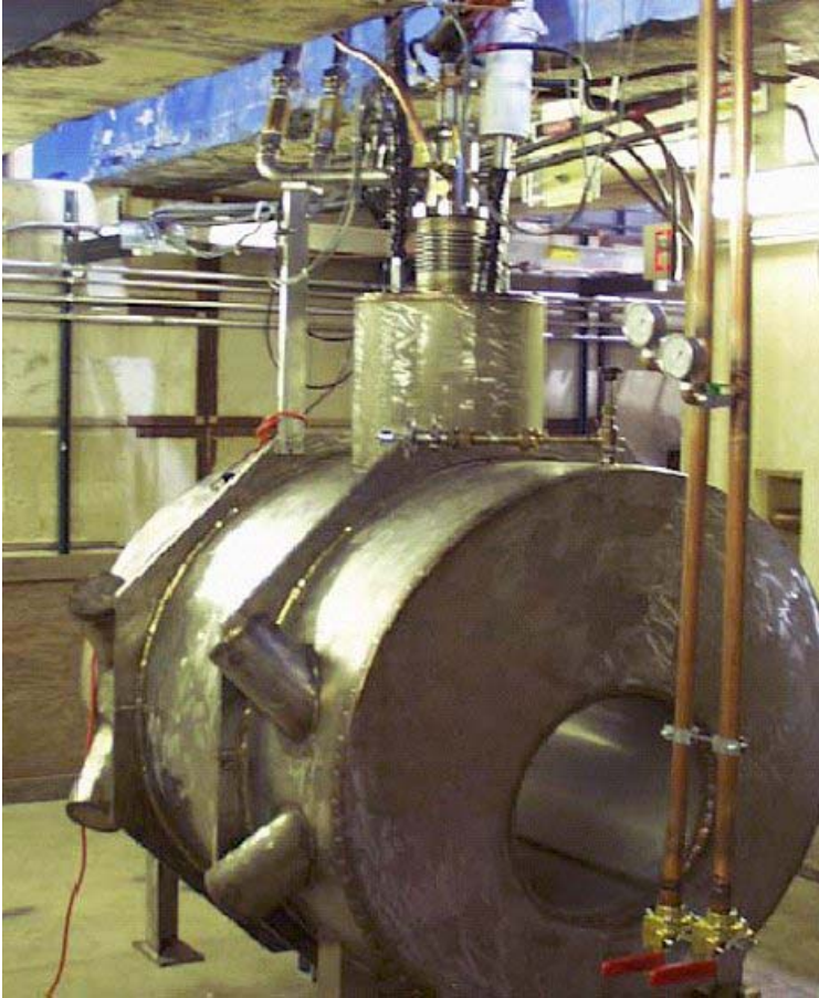
Lab G RF Cave showing 5T SC Magnet 44 cm bore
