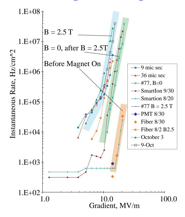
They stayed high when the magnet was turned off, although a long period of conditioning seemed to heal the damage.
