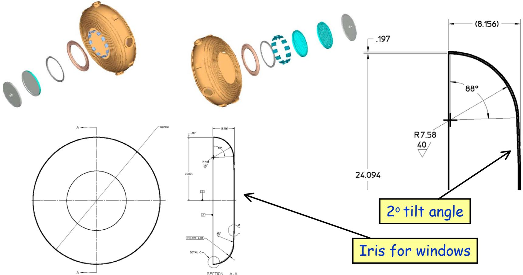
~ 6 mm Cu plates, spinning + e-beam welding
