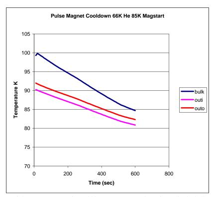
66K inlet temperature, Dtime=.0001 sec - Energy Balance is good. The bulk temp is computed at a mid-axial slice
