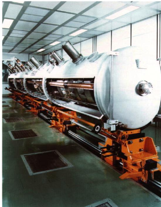
Figure 8.31: LEP cryomodule.
