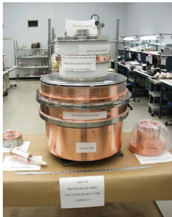
Figure 14.8: 1 MW cw HOM-IOT.
