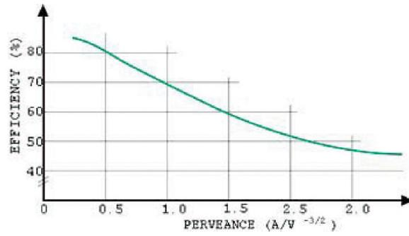
Figure 14.7: Klystron efficiency *vs.* beam perveance.
