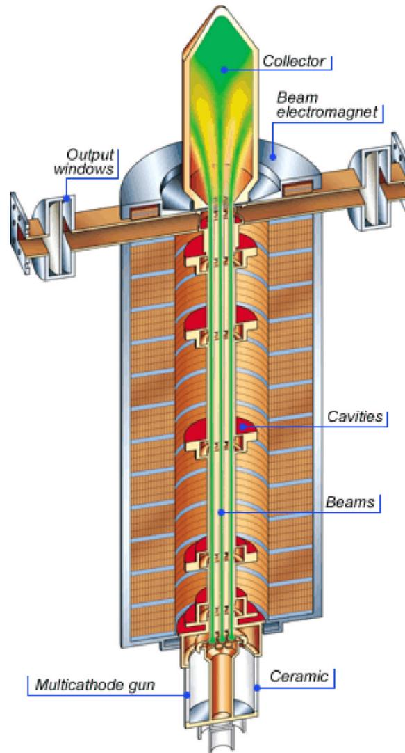
Figure 14.4: Schematic of multi-beam klystron.
