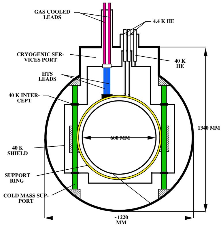
Figure 10.3: Induction cell solenoid cold mass support system and leads.
