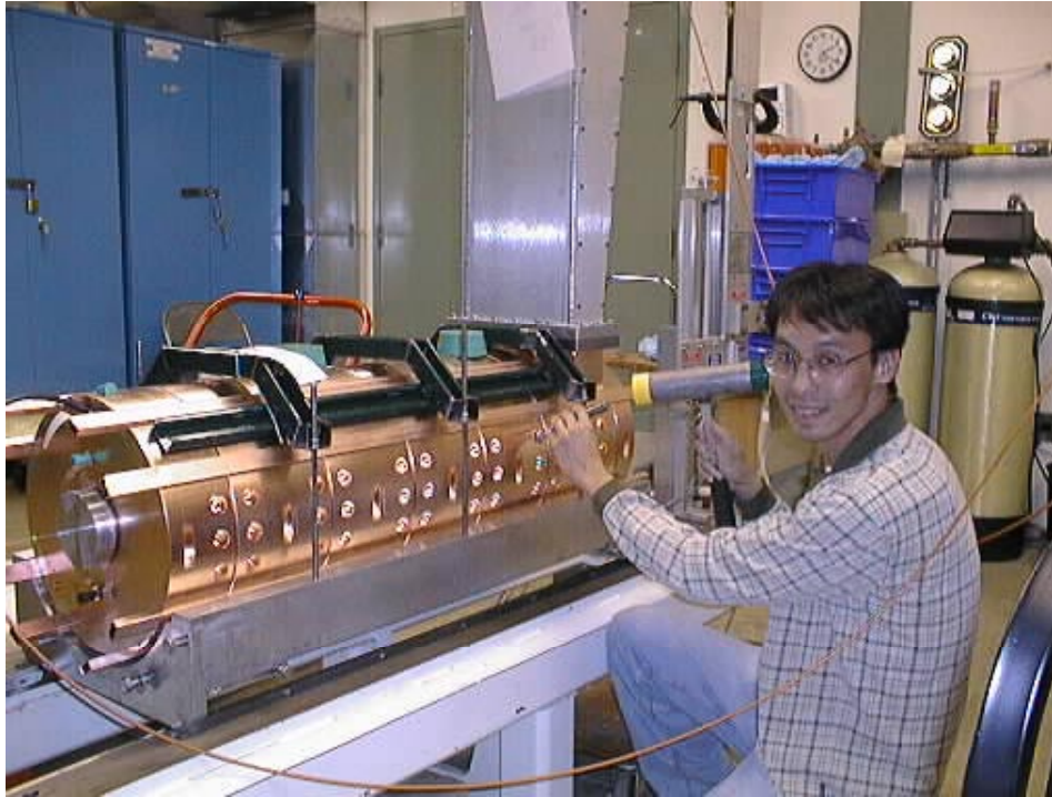
Open-cell cavity being tuned (Fermilab)
