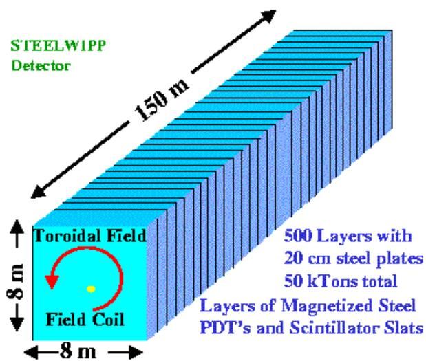
Figure 4.13: A possible 50-kton steel-scintillator-PDT detector at WIPP.
