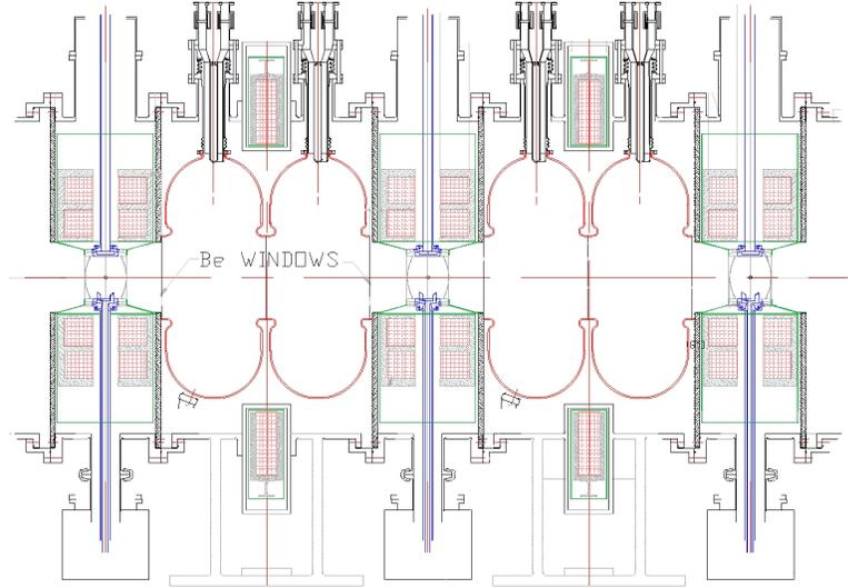
Figure 4.5: Cooling channel Lattice 2, two cavities per cell.
