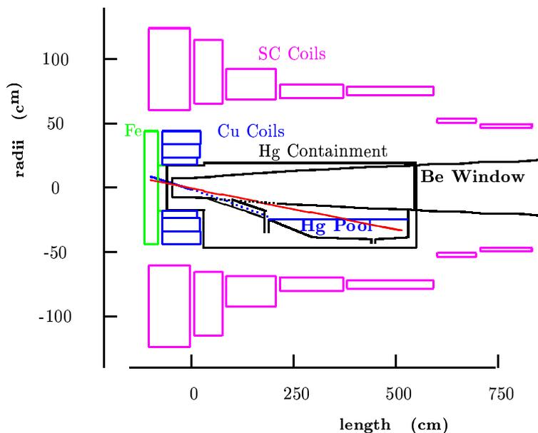
Figure 4.3: Target, capture solenoids and mercury containment.
