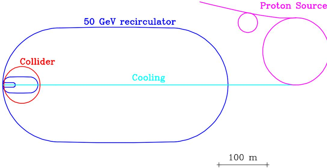
Figure 5.3: Plan of a 0.1-TeV-CoM muon collider.
