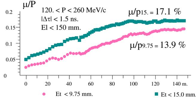
Figure 4.7: Geant4 simulations of the muon-to-proton yield ratio for two transverse emittance cuts, clearly showing that the channel cools, *i.e.*, the density in the center of the phase space region increases. Since the relevant yield  $\mu/p_{15}$  no longer increases for  $z \leq 110$  m, the channel length was set to 108 m.
