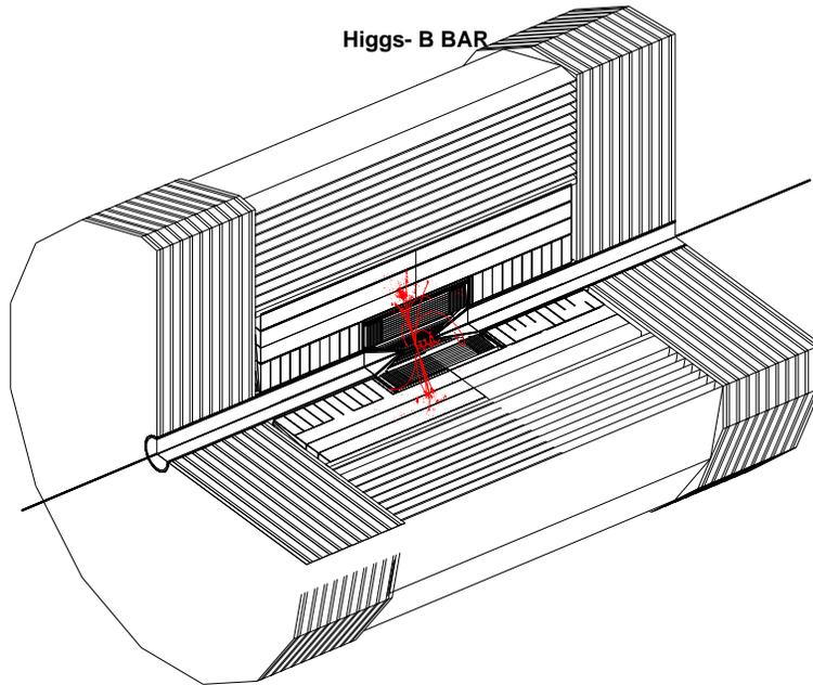
Figure 5.7: Cut view of a strawman detector in GEANT for the Higgs factory with a  $\text{Higgs} \rightarrow b\bar{b}$  event superimposed. No backgrounds shown. The tungsten cones on either side of the interaction region mask out a 20deg area.
