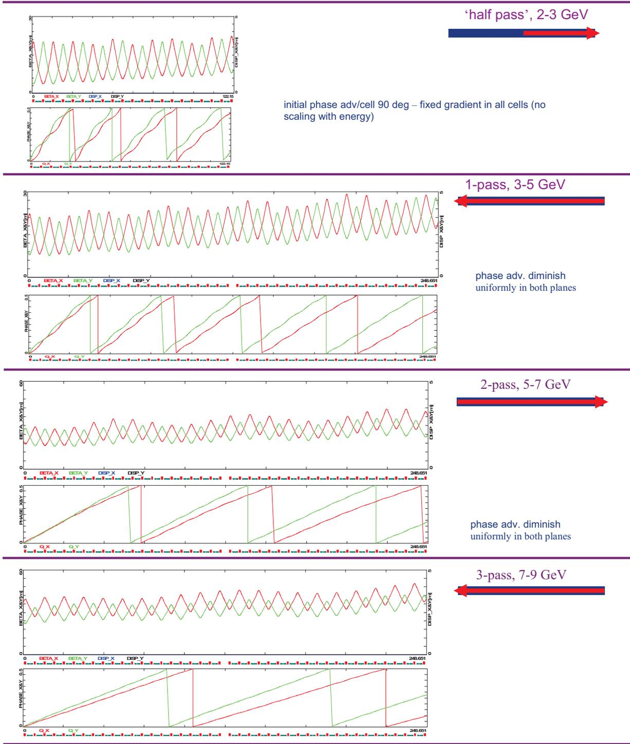
Fig. 45. FODO based multi-pass linac optics for passes 1–3. Quadrupoles in all cells are set to the same gradient, corresponding to  $90^\circ$  phase advance per cell at 2 GeV. Intrinsic to the FODO focusing symmetry between the horizontal and vertical planes, the betatron phase advances gradually diminish uniformly in both planes. The resulting linac optics is well balanced in terms of Twiss functions and beam envelopes, and there is sufficient phase advance for up to six passes.
