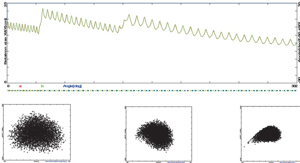
Fig. 38. Top, transverse beam envelopes in the pre-accelerator linac, which has uniform periodic focusing with three styles of cryo-modules. Below, longitudinal phase-space: before, halfway through, and at the end of acceleration, as obtained by particle tracking.
