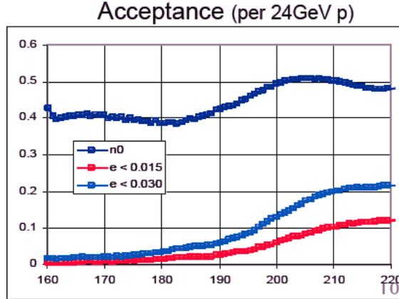
Fig. 36. Accepted number of muons per incident proton as a function of distance in the gas-filled cooling channel. The upper (dark blue) curve is the total number of  $\mu/p$ , the middle (light blue) curve is  $\mu/p$  into the ISS acceptance, and the bottom (red) curve is  $\mu/p$  into the Study 2 acceptance.
