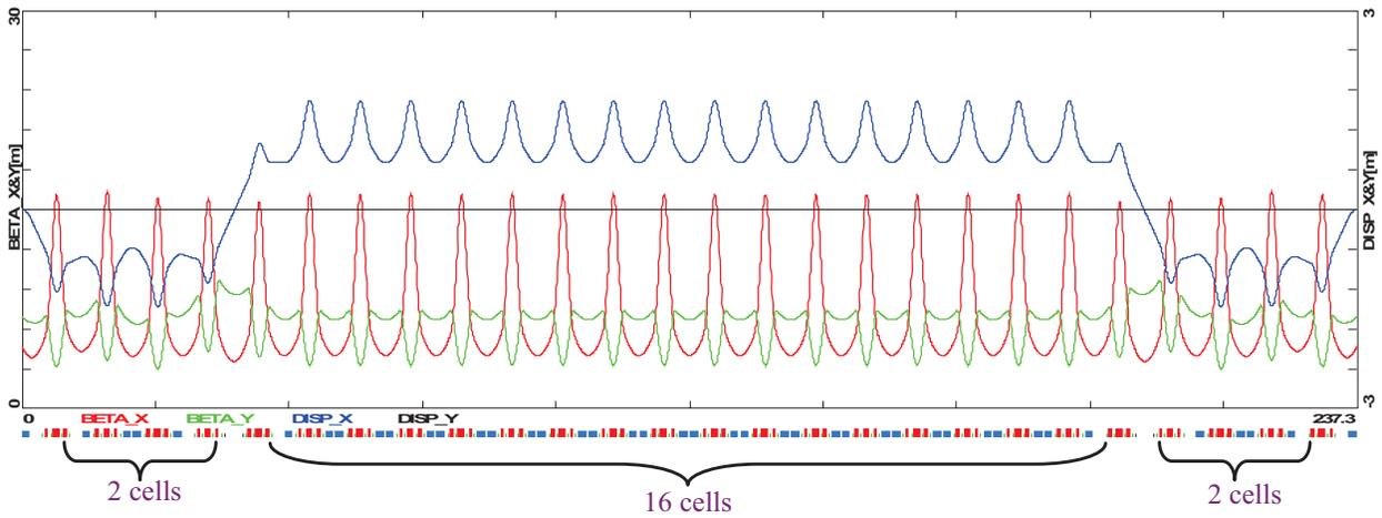
Fig. 48. Droplet arc optics, showing uniform periodicity of beta functions and dispersion.
