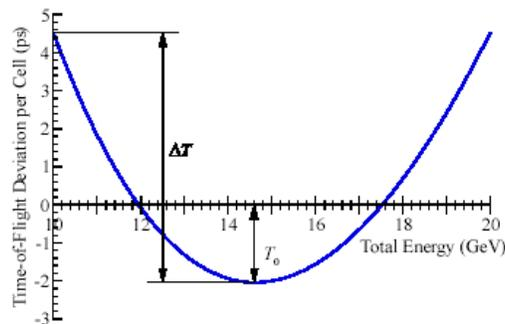
Fig. 52. Time-of-flight as a function of energy in a linear, non-scaling FFAG cell.
