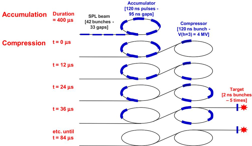
Fig. 9. Accumulation and compression scheme for linac-based proton driver.
