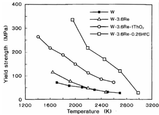
Fig. 17. Yield strength of tungsten and some of its high-strength alloys.
