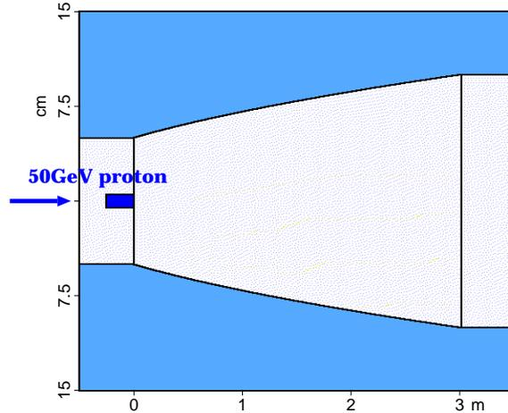
Fig. 20. Capture system from Ref. [32], comprising a 20 T solenoid followed by a rapid taper to 5 T.
