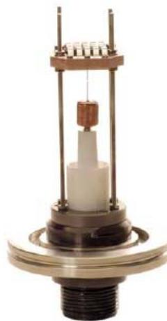
Fig. 14. Wire test assembly.
