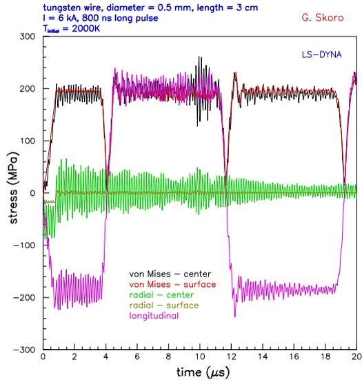
Fig. 16. Typical radial stress in the tungsten wire from thermal and Lorentz forces.
