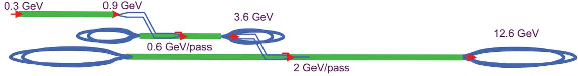
Fig. 41. Layout of two-step dogbone RLA complex. For compactness, all three subsystems (pre-accelerator, dogbone I and dogbone II) are stacked up vertically;  $\mu^\pm$  beam transfer between the accelerator components is facilitated by the vertical double chicane (see text).
