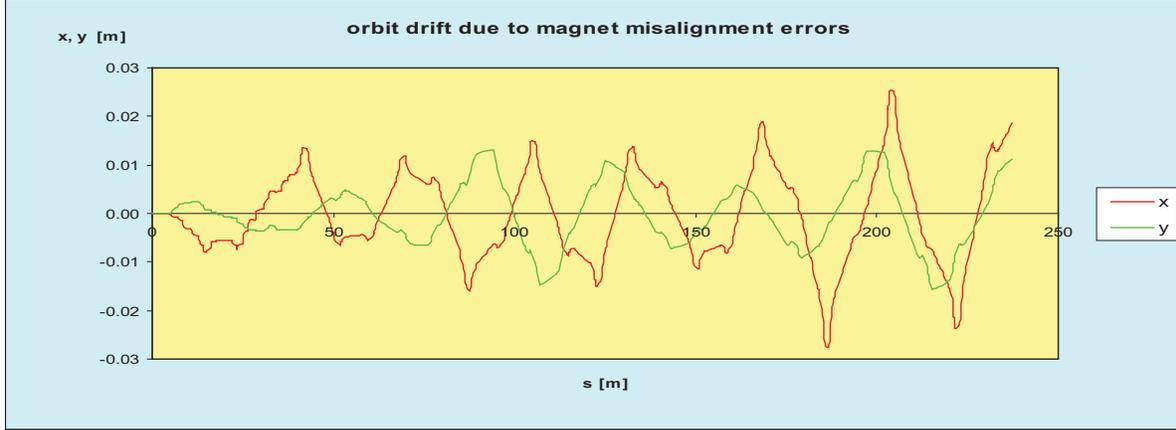
Fig. 51. Orbit deviation due to magnet misalignment errors.
