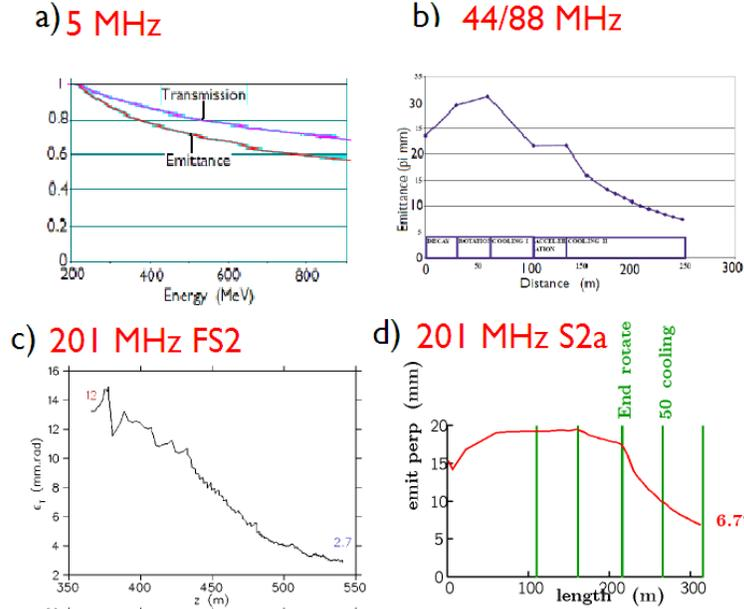
Fig. 29. Emittances vs. distance along cooling channel: a) 5 MHz in an FFAG; b) 44 and 88 MHz tapered system; c) Study 2 tapered system at 201 MHz; d) Study 2a non-tapered system. In a), “distance” is represented in units of the beam energy after some number of turns in the ring.
