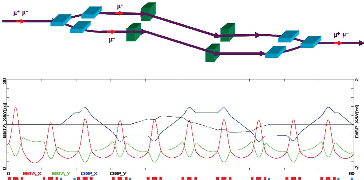
Fig. 50. Layout and optics of the injection double chicane.
