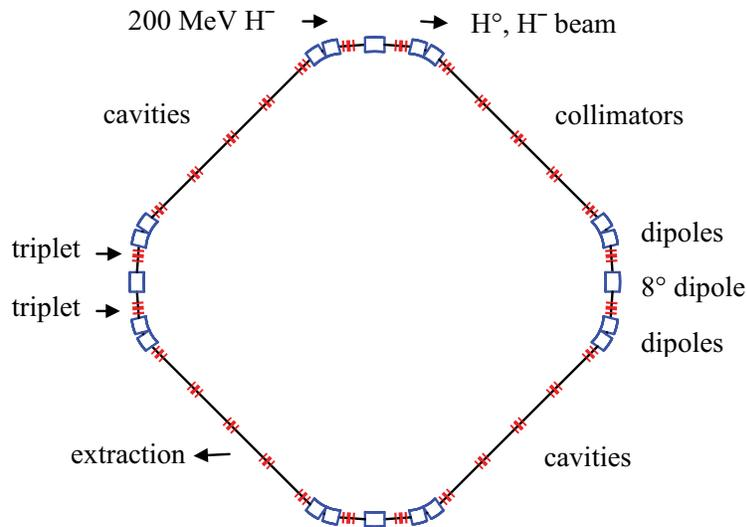
Fig. 3. Layout of 50 Hz, 3 GeV booster synchrotron.
