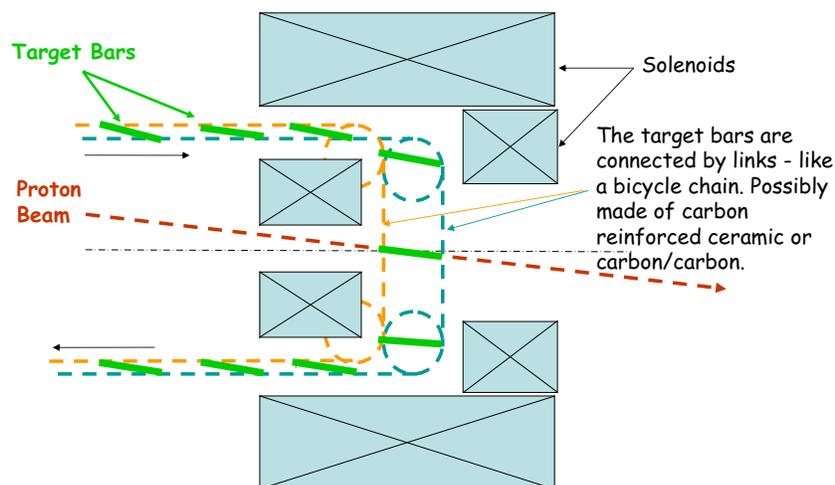
Fig. 12. Schematic diagram of a solid target scenario.
