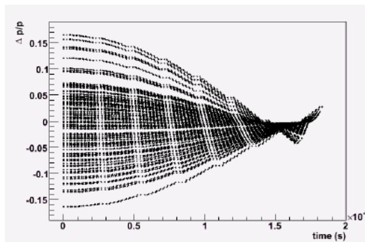
Fig. 35. Energy spread of Gaussian beam versus time in the simulation model of PRISM.
