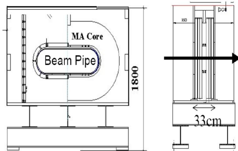
Fig. 23. 5 MHz ferrite-loaded cavity for FFAG scheme.
