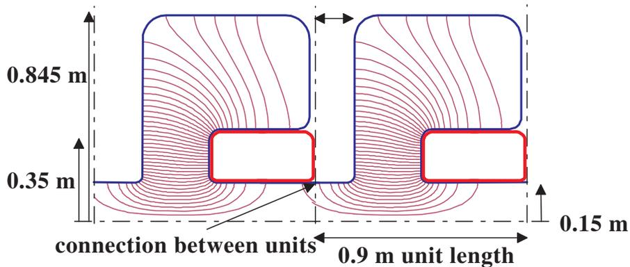
Fig. 24. 88 MHz vacuum cavity with integrated solenoids.
