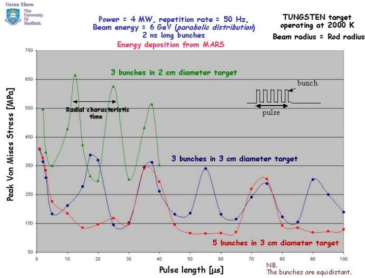
Fig. 15. Thermal stress as a function of target diameter, number and spacing of proton bunches in a macro-pulse.
