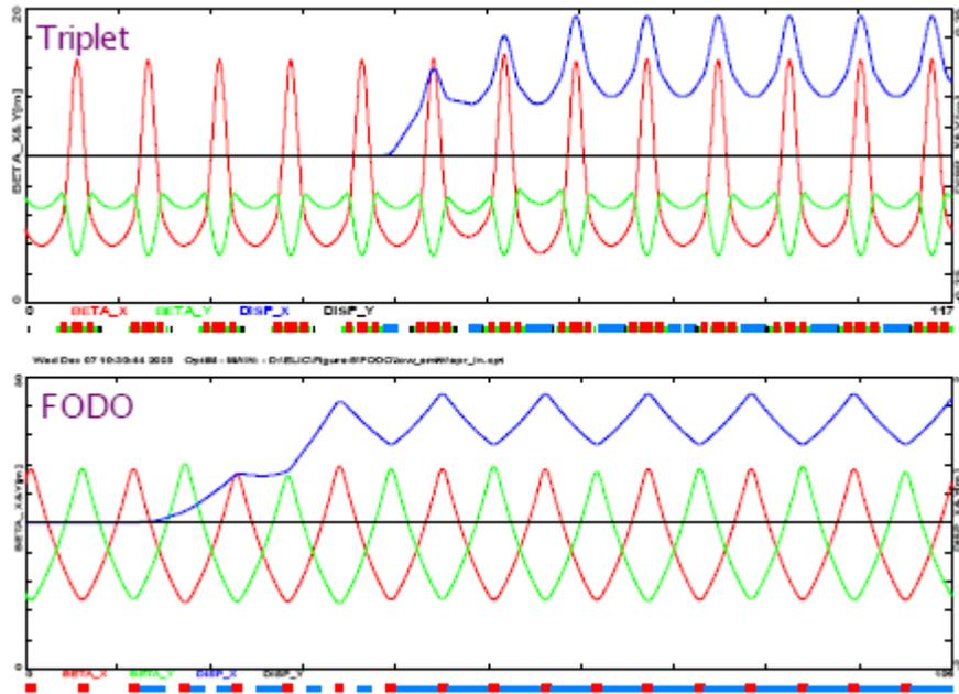
Fig. 49. Spreader optics showing uniform periodicity of beta functions and dispersion. These optics apply to either the FODO or the triplet design.
