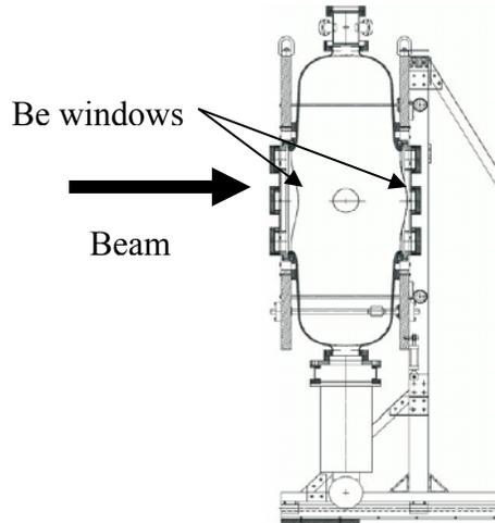
Fig. 25. 201 MHz test cavity, showing mounting arrangement. The ports on the entrance and exit faces are for diagnostic purposes. The curved surfaces represent thin Be windows that electrically close the irises.
