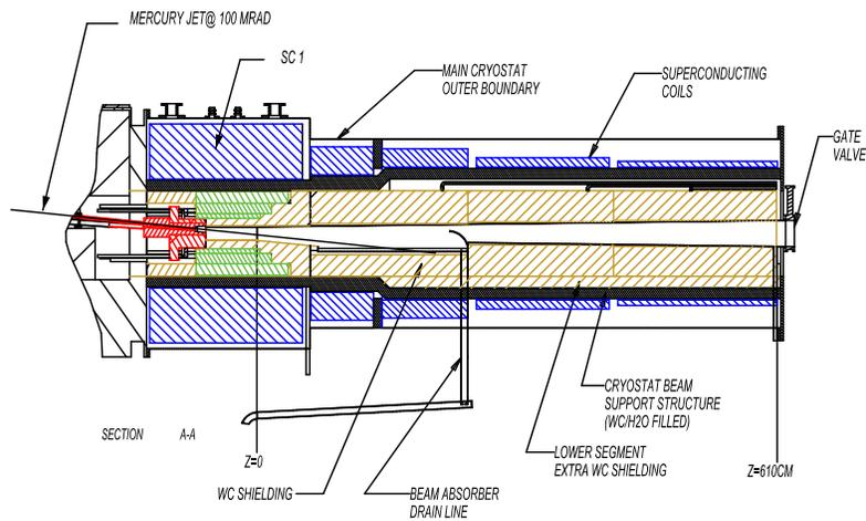
Fig. 18. Baseline ISS target system. The solenoidal field at the target position is 20 T. The downstream coils begin the process of adiabatically tapering the field to 1.75 T for further transport.
