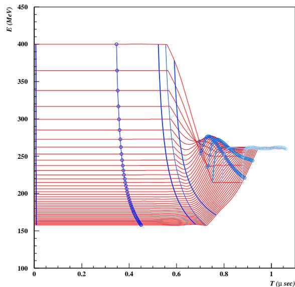
Fig. 34. Energy of a set of test particles as a function of time in the phase rotation channel.
