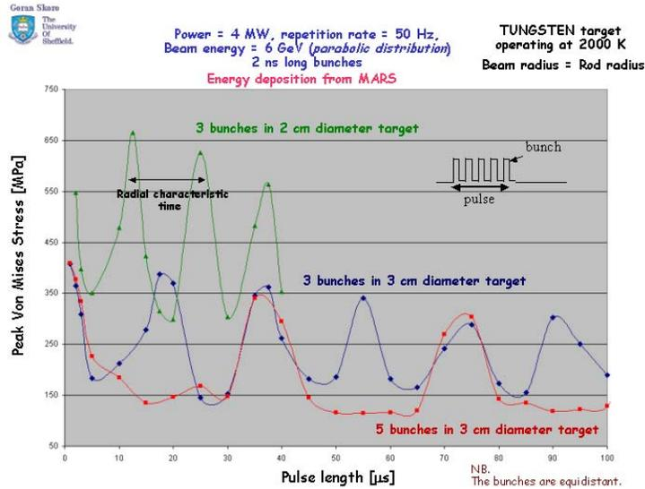
Fig. 15. Thermal stress as a function of target diameter, number and spacing of proton bunches in a macro-pulse.
