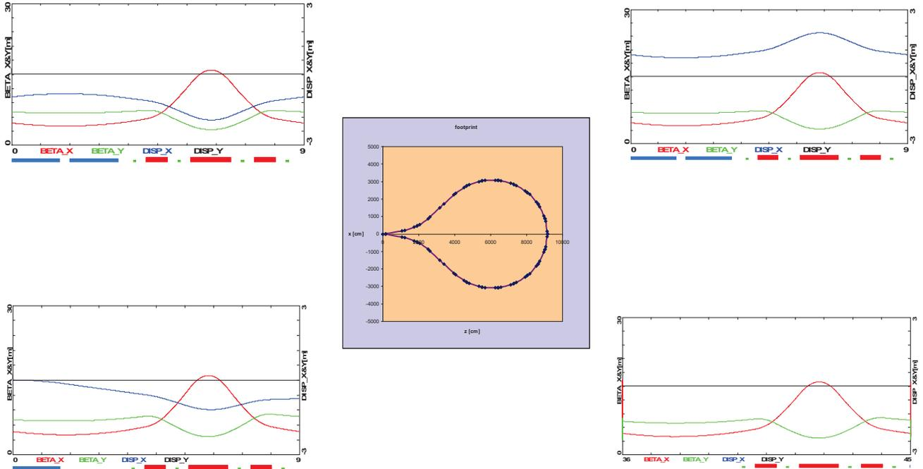
Fig. 47. The lattice building blocks: triplet  $90^\circ$  phase advance cells; inward and outward cells, missing dipole empty cells.
