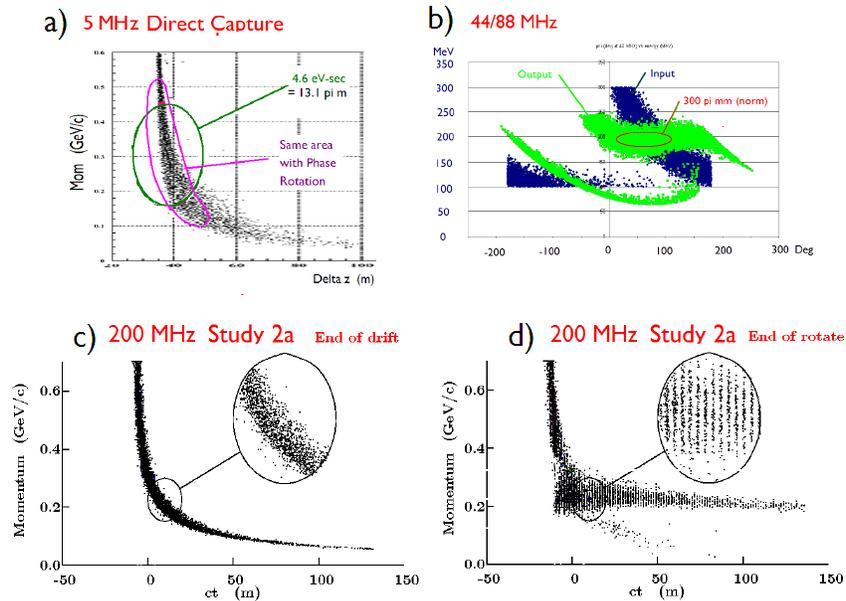
Fig. 27. Phase-space plots of phase rotation cases: a) 5 MHz before rotation with captured ellipses without rotation (green), and with rotation (magenta); b) CERN 44 MHz, before (blue) and after (green) rotation with eventual 88 MHz acceptance in red; c) and d) Study 2a before and after rotation.
