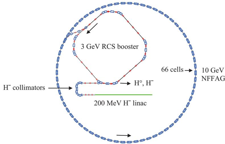
Fig. 6. Schematic layout drawing of the linac, booster and NFFAG of the proton driver.
