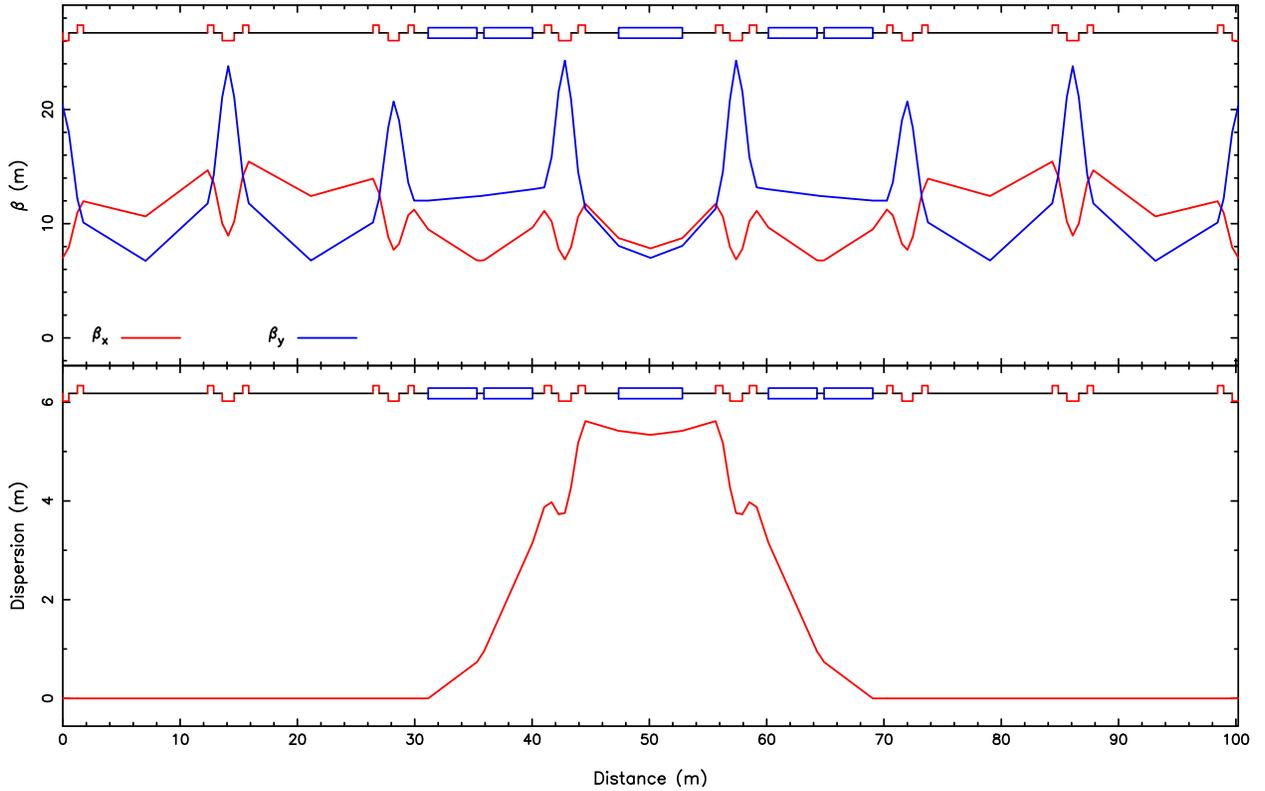
Fig. 4. (upper) Betatron functions for the 400.8 m booster synchrotron; (lower) booster dispersion function.
