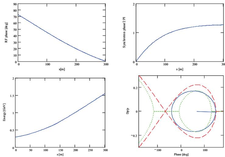
Fig. 39. Individual cavity phasing along the linac and the resulting synchrotron motion. The energy profile and the longitudinal beam boundary (solid line) inside a separatrix (dashed line) are shown at the beginning of the linac ( $\Delta p/p = \pm 0.17$  or  $\Delta\phi = \pm 92^\circ$ ).
