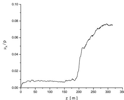
Fig. 32. Number of muons per incident proton accepted by the downstream acceleration system vs. longitudinal position along the ISS front end. The cooling channel begins at 216 m in this plot. Note that some increase in accepted muons takes place in the phase rotation section upstream of the cooling channel, where more particles are moved into the energy acceptance of the acceleration system.
