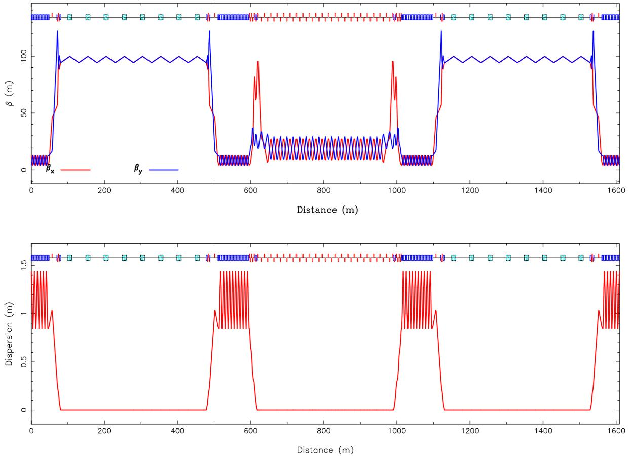
Fig. 61. Lattice betatron (top) and dispersion (bottom) functions for the 1608.8 m, triangle decay rings.
