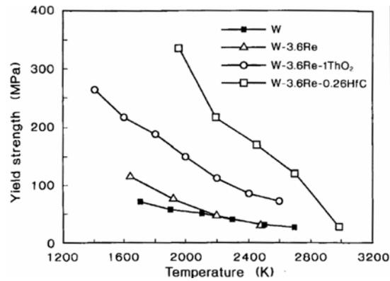
Fig. 17. Yield strength of tungsten and some of its high-strength alloys.
