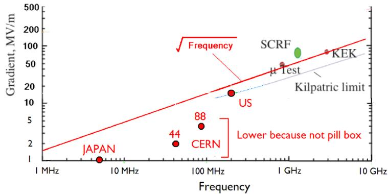
Fig. 26. Gradients vs. frequency.
