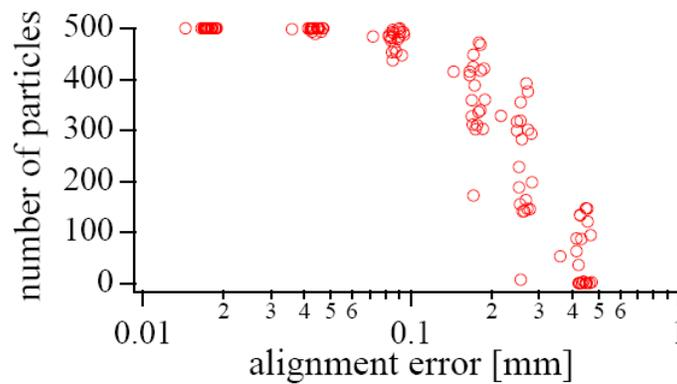
Fig. 57. Number of surviving particles as a function of alignment error.
