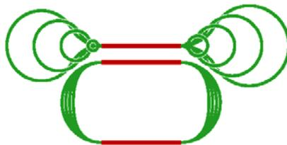
Fig. 40. RLA geometries: dogbone layout (above), racetrack layout (below).
