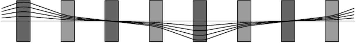
Fig. 55. Trajectories in a FODO lattice, demonstrating that path lengths are longer for particles with larger transverse amplitude.
