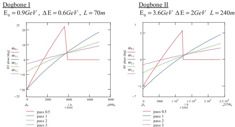
Fig. 42. RF phase slippage along the multi-pass linacs; initial ‘gang phases’ for each pass were chosen for optimum longitudinal bunch compression in each linac-arc segment. For dogbone 1, the gang phases were  $-20^\circ$ ,  $-20^\circ$ ,  $-8^\circ$ , and  $-3^\circ$ , respectively, for the four passes through the device; for dogbone 2, the gang phases were  $-5^\circ$ ,  $-5.5^\circ$ ,  $-2.5^\circ$ , and  $-1^\circ$ , respectively, for the four passes.
