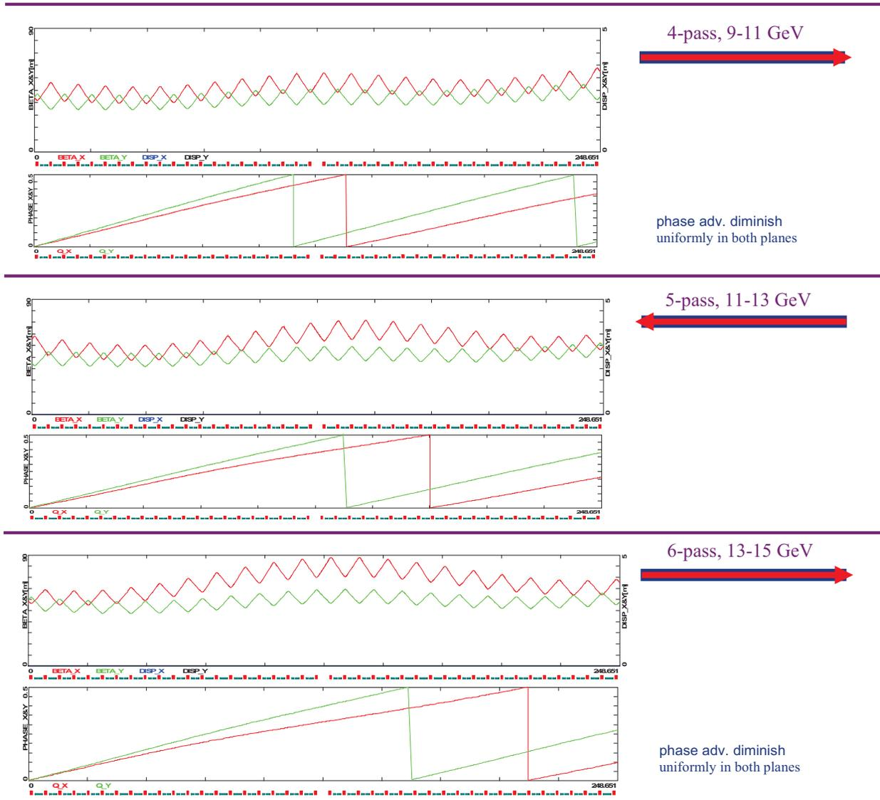
Fig. 46. FODO based multi-pass linac optics for passes 4–6. Quadrupoles in all cells are set to the same gradient, corresponding to  $90^\circ$  phase advance per cell at 2 GeV. Intrinsic to the FODO focusing symmetry between the horizontal and vertical planes, the betatron phase advances gradually diminish uniformly in both planes. The resulting linac optics is well balanced in terms of Twiss functions and beam envelopes, and there is sufficient phase advance for up to six passes.
