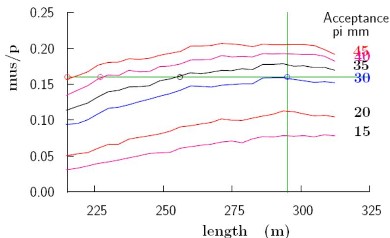
Fig. 30. Accepted number of muons per proton as a function of distance along the cooling channel for various assumed downstream accelerator transverse acceptances. The cooling channel begins at 216 m in the length coordinate plotted.
