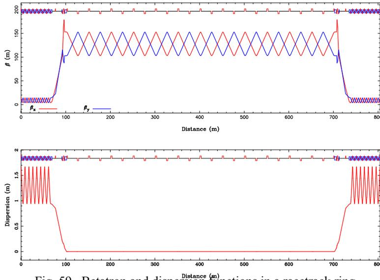
Fig. 59. Betatron and dispersion functions in a racetrack ring.
