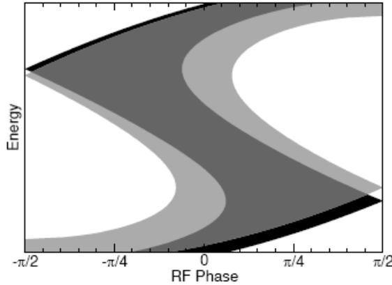
Fig. 54. Phase space channel for low amplitude particles (black) and high amplitude particles (light grey). The overlap region is dark grey. Particles start at low energy (bottom) and are accelerated to high energy (top).
