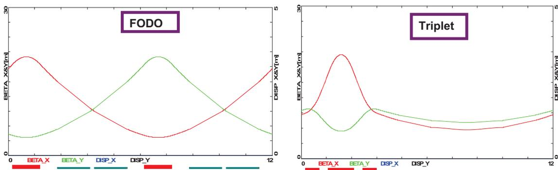
Fig. 43. Comparison of FODO and triplet focusing structures. Both designs use the same cell length (12 m) and betatron phase advance per cell ( $90^\circ$ ).
