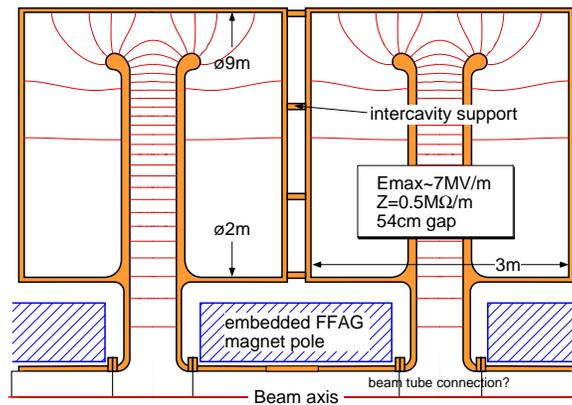
Fig. 22. 5 MHz vacuum cavity for FFAG scheme.
