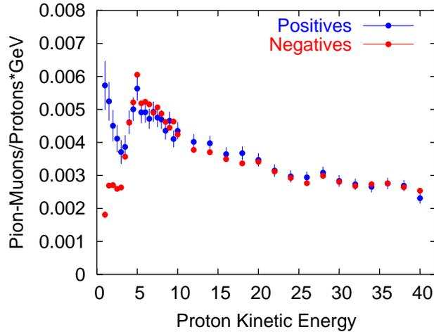
Fig. 11. Calculated production efficiency for a carbon target. The yield per proton and per GeV is lower than for a mercury target and peaks at a lower energy.
