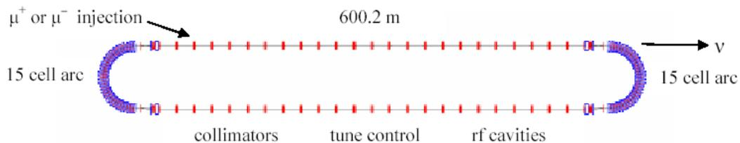
Fig. 58. Schematic layout for a racetrack shaped, muon decay ring.
