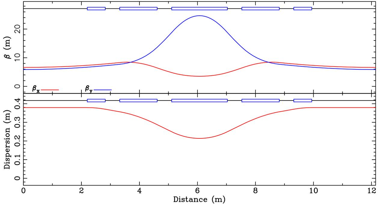
Fig. 7. Small amplitude betatron (top) and dispersion (bottom) functions for the NFFAG 10 GeV orbit.
