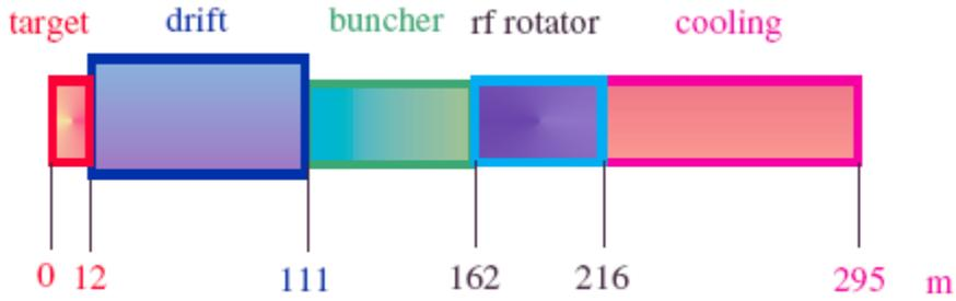
Fig. 31. Schematic layout of ISS baseline front end.
