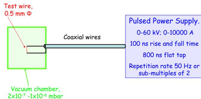
Fig. 13. Schematic diagram of the test wire and power supply.
