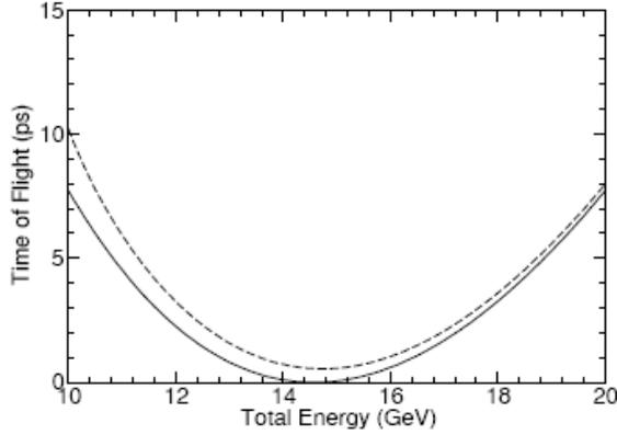
Fig. 53. Time-of-flight as a function of energy for zero transverse amplitude (solid) and  $30 \pi$  mm-rad (dashed) normalized transverse amplitude (twice the transverse action, normalized).
