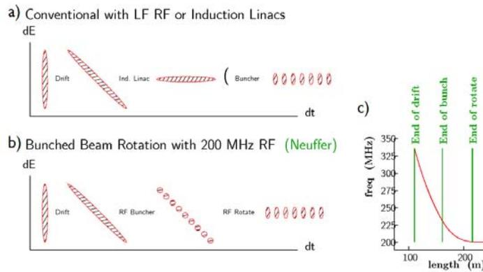
Fig. 19. Phase rotation methods: a) conventional; b) Neuffer bunched beam phase rotation. c) Shows frequency vs. distance for the case of Study 2a, a version of b).
