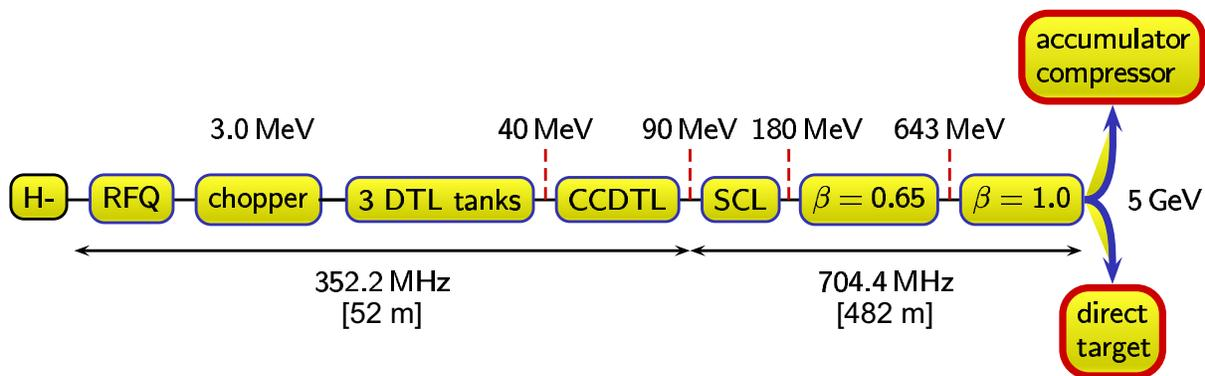
Fig. 8. SPL block diagram.
