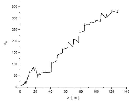
Fig. 33. Number of muons in the accelerator acceptance vs. distance along the CERN channel.
