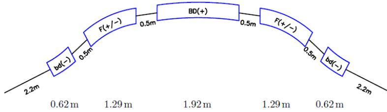
Fig. 5. A single lattice cell of the 50 Hz, 4 MW, 10 GeV, NFFAG proton driver ring.
