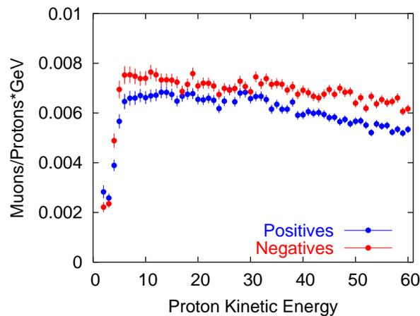
Fig. 10. Calculated production efficiency of positive and negative muons at the end of the Study 2a cooling channel, per proton and per GeV of proton beam energy, for a mercury-jet target. Although the curves are rather flat, an optimum energy, roughly 10 GeV, is discernible. Below about 5 GeV, the calculations show an abrupt fall-off in production. Above 10 GeV the fall-off is small but, from the muon production perspective, there is no benefit to increasing the beam energy beyond 10 GeV.
