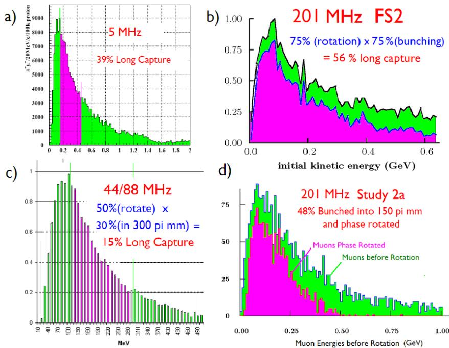
Fig. 28. Momentum ranges captured by various phase rotation systems: a) 5 MHz without phase rotation; b) induction linac system; c) 44 MHz rotation; d) 201 MHz bunched beam phase rotation.
