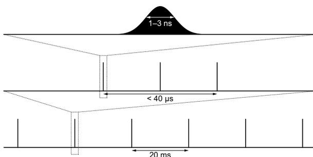
Fig. 1 Proton bunch structure. The top picture represents a single proton micro-bunch, the middle picture shows the spacing of three such micro-bunches that hit the production target in one proton driver cycle, and the bottom picture shows the overall 50 Hz repetition rate of the proton driver.
