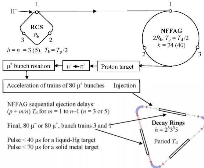
Fig. 2. Bunch patterns ( $n = 3$ ) for the proton driver and decay rings. This example assumes triangular decay rings.
