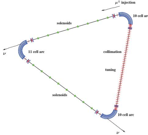
Fig. 60. Schematic layout for a  $52.8^\circ$  apex angle, isosceles triangle, muon decay ring.
