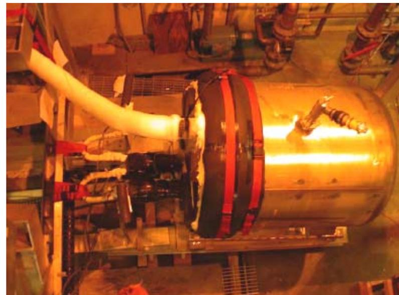
15-T solenoid during tests at MIT
