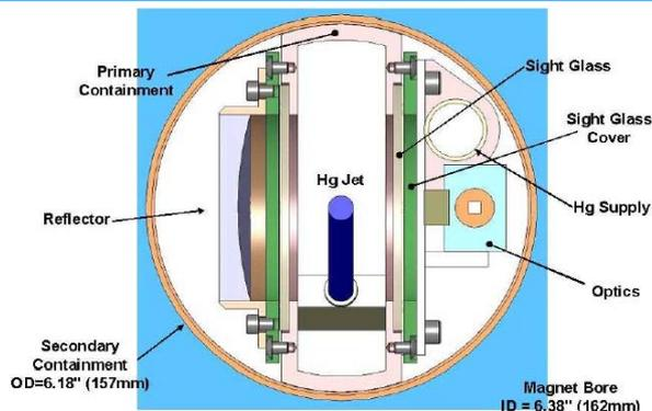
Hg delivery and containment system under construction at ORNL. Integration tests scheduled this Fall at MIT.
