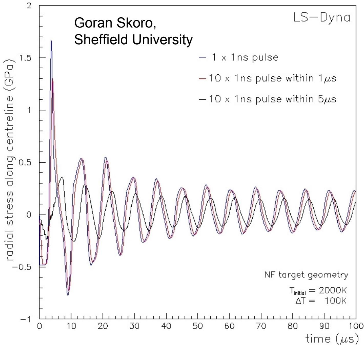
Effect of 10 micro-pulses in 1 and 5  $\mu\text{s}$  long macro-pulses.
