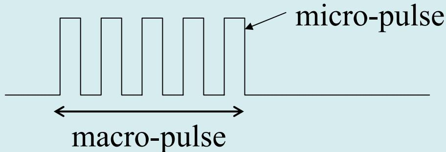
Proton beam "macro-pulses" and "micro-pulses".
