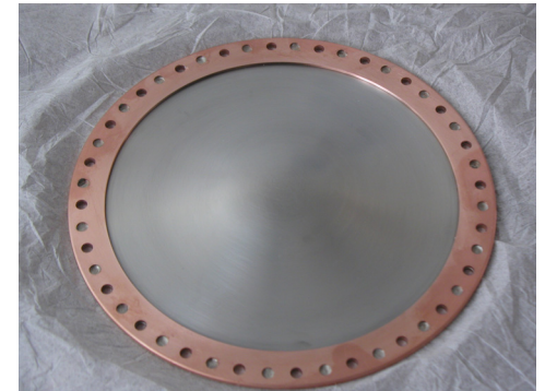
201MHz RF cavity with beryllium windows
