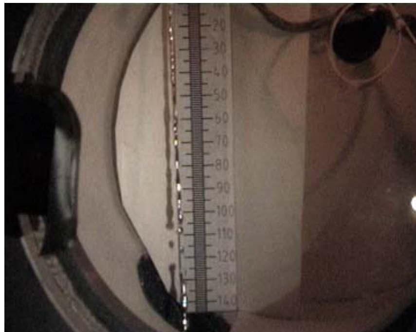
Liquid Gallium jet in the cross section of the discharge chamber at different velocity of issue. The below photo displays a phenomenon of jet disintegration (diameter of jet \varnothing 2.3 mm)
