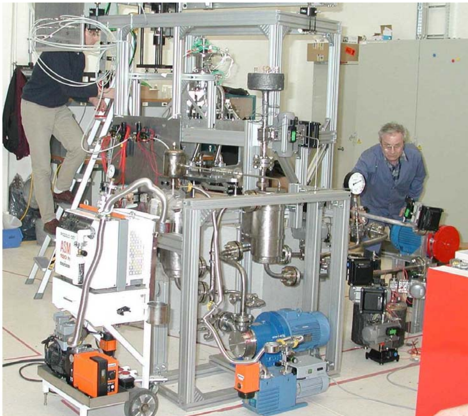
Lead bismuth eutectic loop for LiSoR facility LBE loop for LiSoR experiment at PSI
