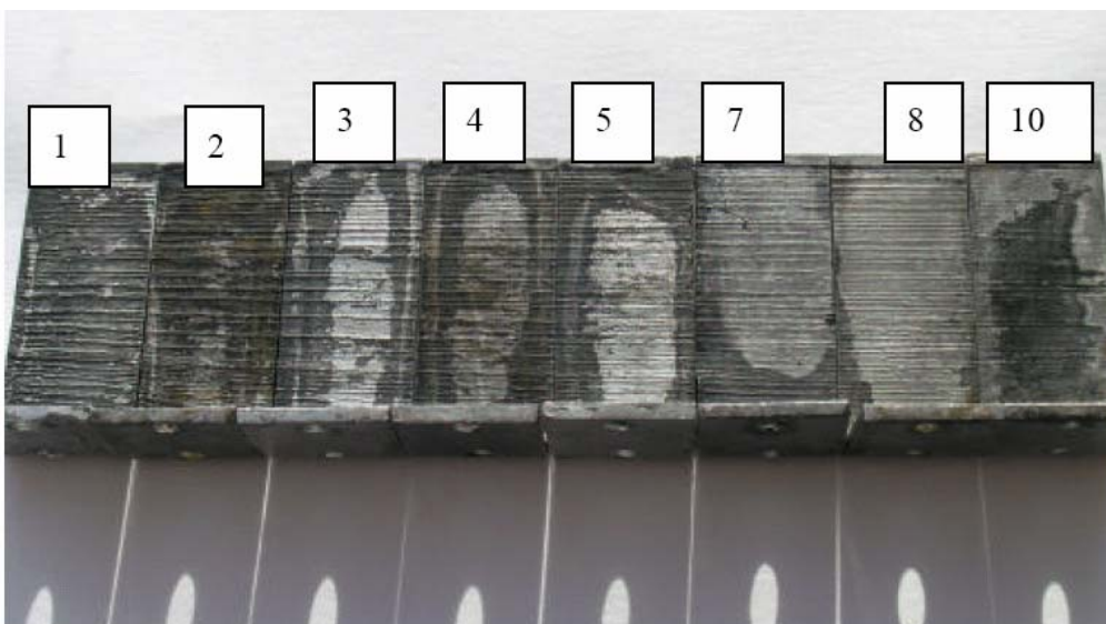
EUROFER steel samples located in zone with magnetic field ( B = 1.7 Tesla)
