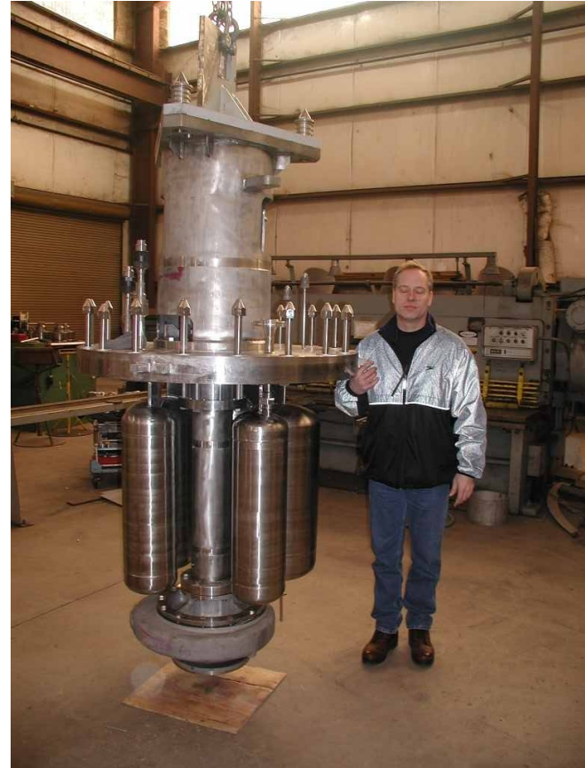
Pump Removed From Vessel
