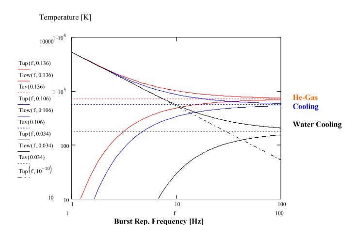
**Table 1:** Minimum and maximum temperature inside spheres and He-gas during the 50 Hz pulsed beam. The time average temperatures refer to a 4 MW continuous beam.
