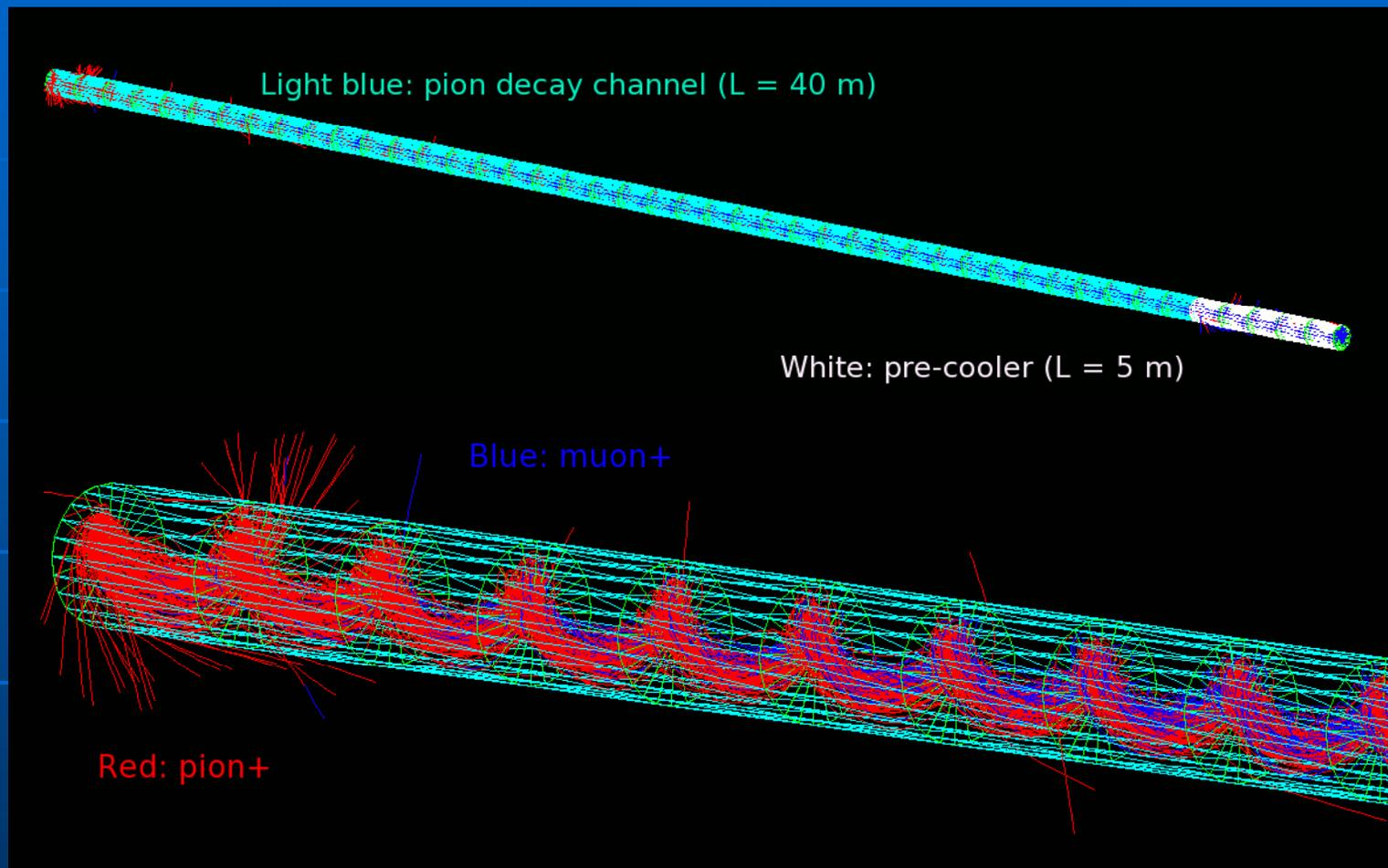
40 m evacuated helical magnet pion decay channel
