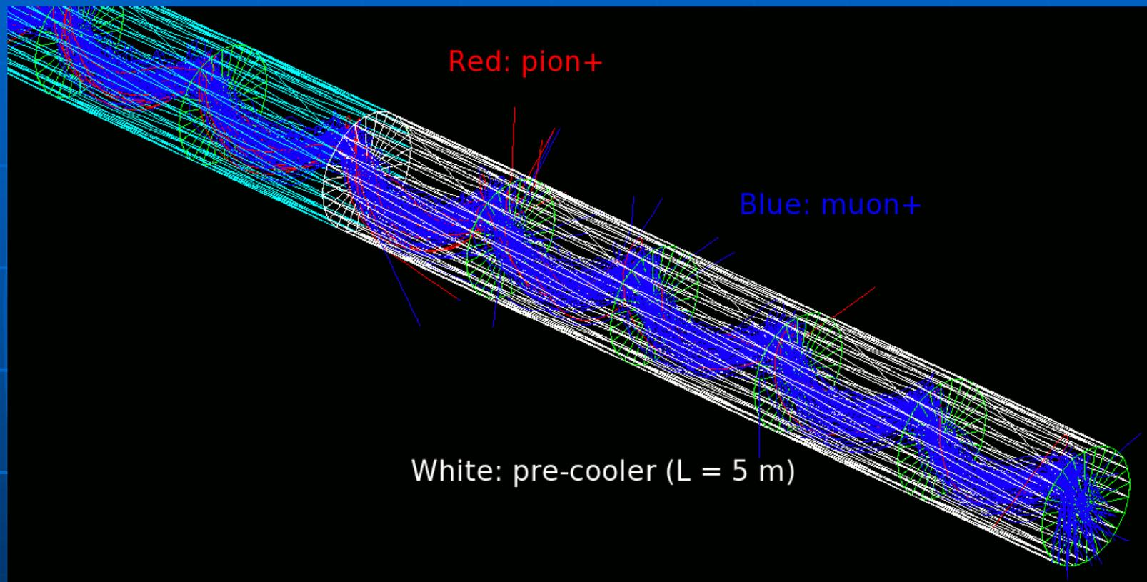
New Invention: HCC with fields that decrease with momentum. Here the beam decelerates in liquid hydrogen (white region) while the fields diminish accordingly.
