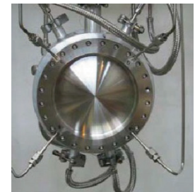
42 cm \varnothing Be RF window
