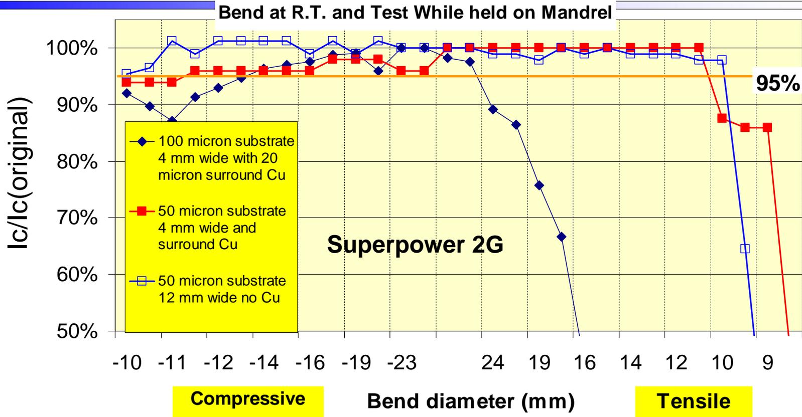
Maximum Bend Strain =  $\pm t / D \sim 95 \mu\text{m} / 11000 \mu\text{m} = 0.86 \%$  ( $\sim 0.45 \%$  on the YBCO)
