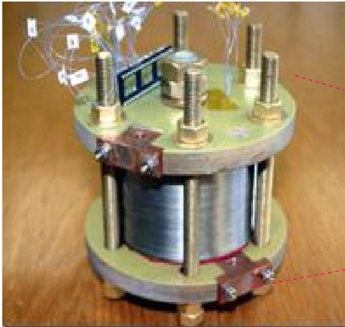
2G HF Insert Coil Showing Terminals, Overbanding and Partial Support Structure. Flange OD is 127 mm.
