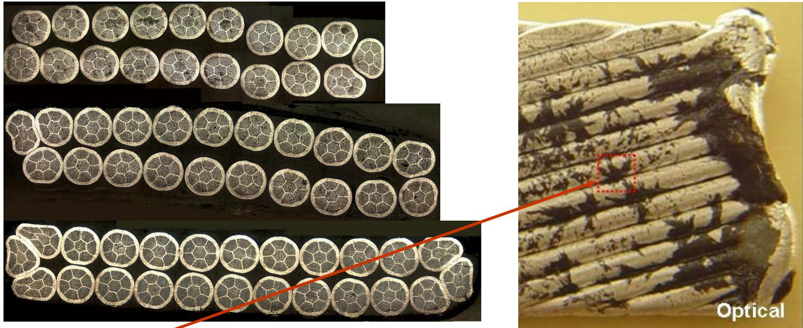
**All cables had black spots after reaction at OST. SEM/EDS analysis showed that the black spots included Bi-2212 and MgO. Half a dozen cables were tested at self-fields of 0.1 to 0.3 T. For all, an  $I_c$  degradation of about 50% was measured. The extracted strands were fine and their degradation was less than 20%.**
