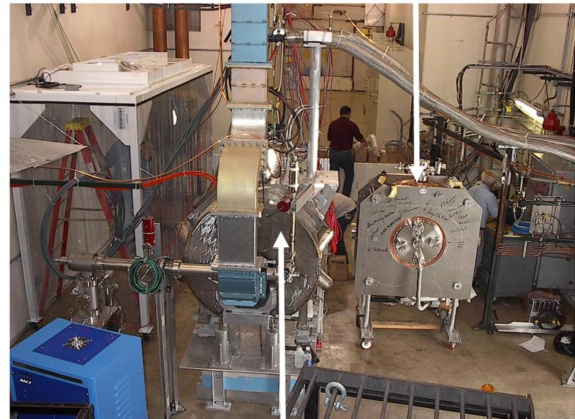
5-T solenoid + 805-MHz cavity
