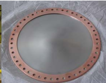
200MHz RF cavity with beryllium windows
