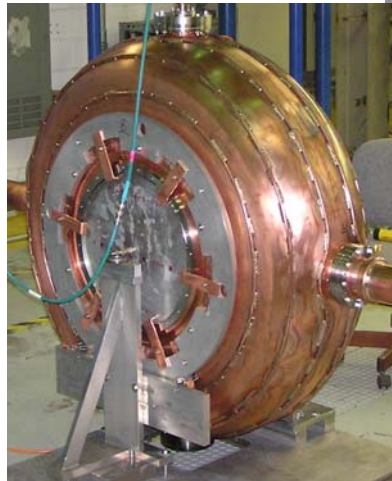
200MHz RF cavity with beryllium windows
