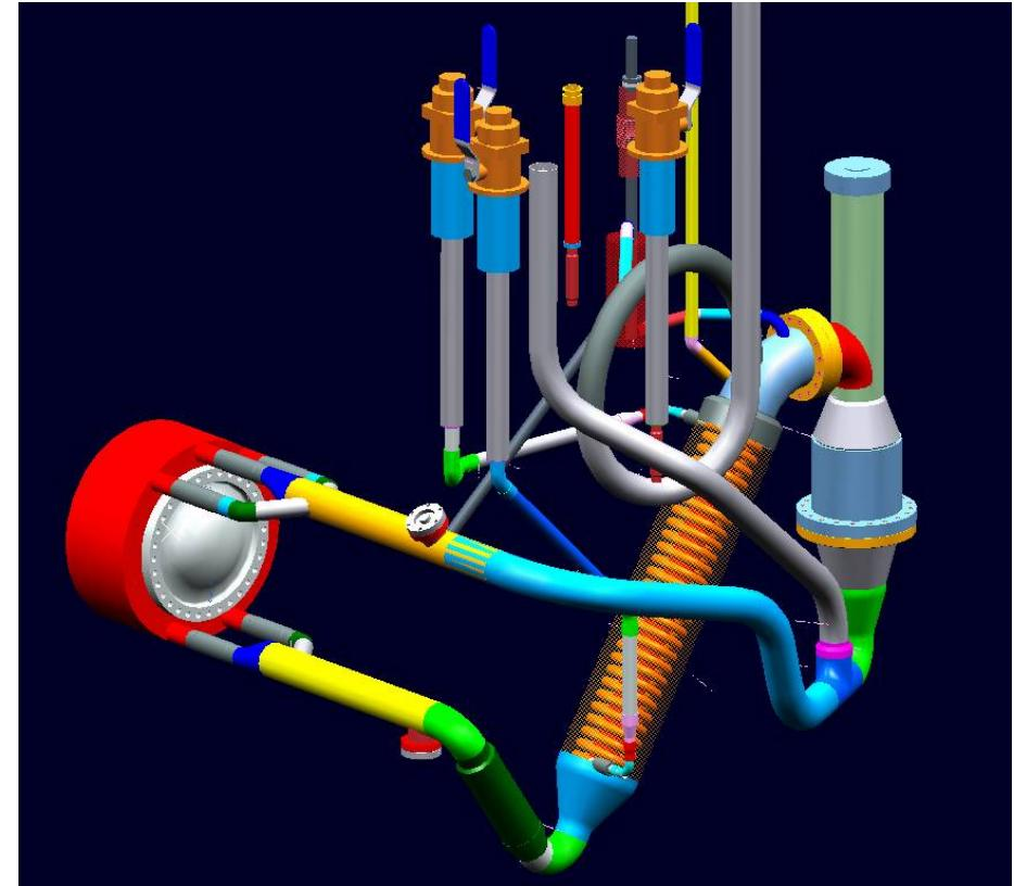
Forced-Flow with external cooling loop
