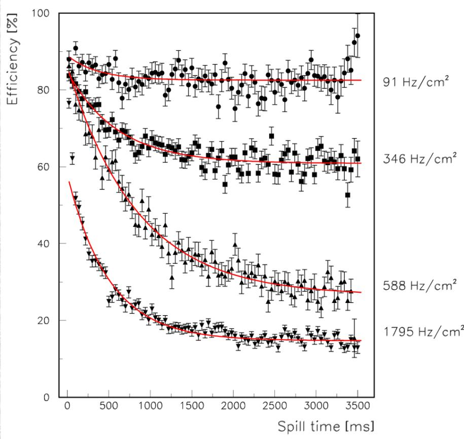
MIP detection efficiency as a function of spill time for various beam intensities. The red curves are fits to the data using the sum of an exponential and a constant.
