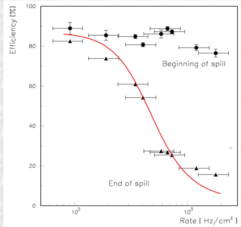
MIP detection efficiency as a function of beam intensity at the beginning (squares) and the end (triangles) of a spill.
