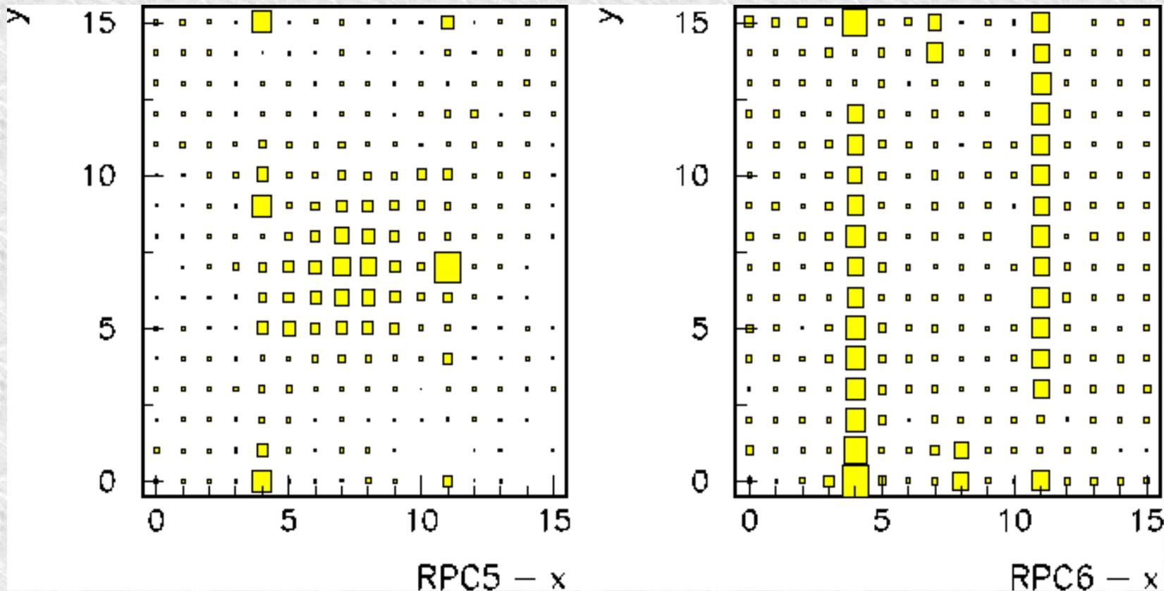
x - y map of the noise hits for a typical default (RPC5) and the 'exotic' (RPC6) chamber. A clear clustering along the fishing lines located approximately at  $x = 4.2$  and  $10.7$  is visible.
