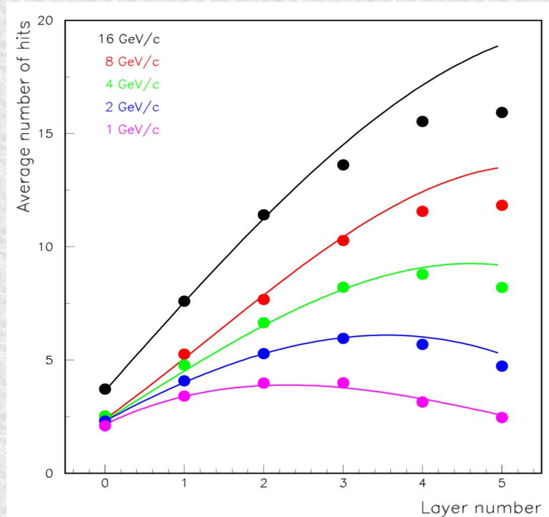
Average number of hits as a function of layer number for the various beam energies. The lines represent the results of a GEANT4 simulation of the set-up together with the simulation of the response of RPCs with a standalone program (RPCSIM by J. Repond).
