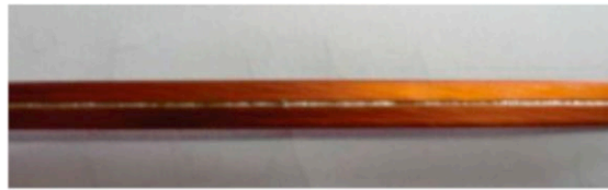
SC joint soldered by ICST, ~1m overlap length, ~1.31nohm at 4.2K and 5T
