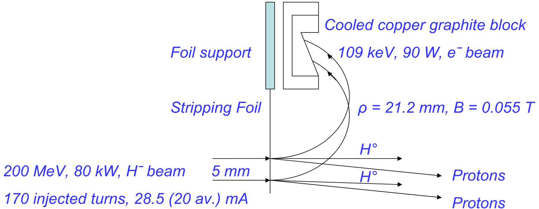
Foil lattice parameters :  $\beta_v = 7.0$  m,  $\beta_h = 7.8$  m,  $D_h = 5.3$  m,  $D_h / \beta_h = 1.93$  m<sup>1/2</sup>
