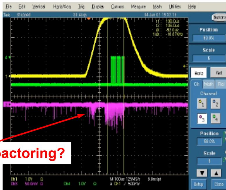
Typical multipactoring waveform pattern observed at the 805 MHz cavity at MTA
