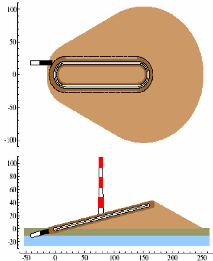
Figure 1.5: Top view and cross section through ring and berm. The 110 m tall tower, drawn to scale, gives a sense of the height of the ring on the BNL landscape.
