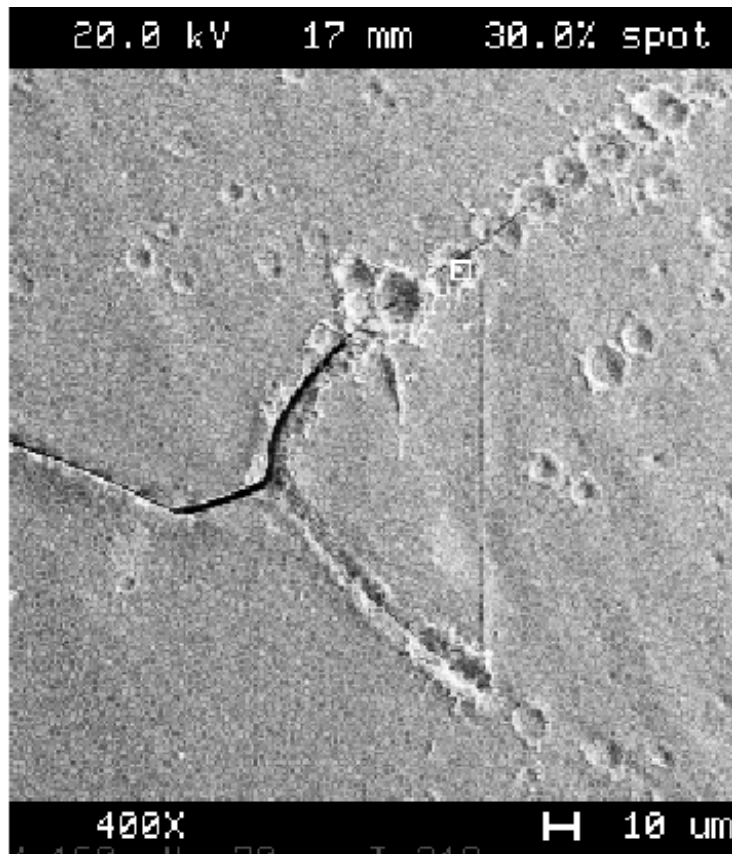
NLC prototype cavity damage
