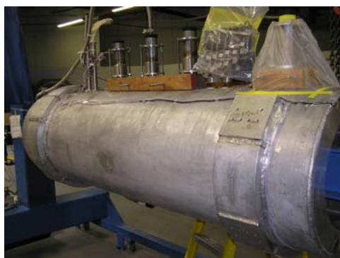
Fig. 7. Preparation of magnet 1 cold mass for reassembly at Wang NMR. Provision for a possible fourth 2-stage cooler is visible in the upper right.
