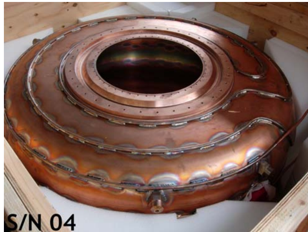
Fig. 9. Completed 201-MHz cavity after acceptance by LBNL.
