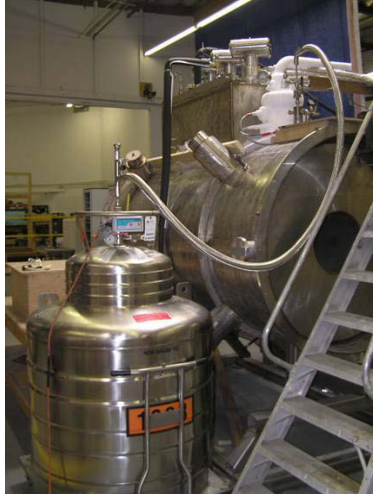
Fig. 6. Second spectrometer solenoid under test at Wang NMR.
