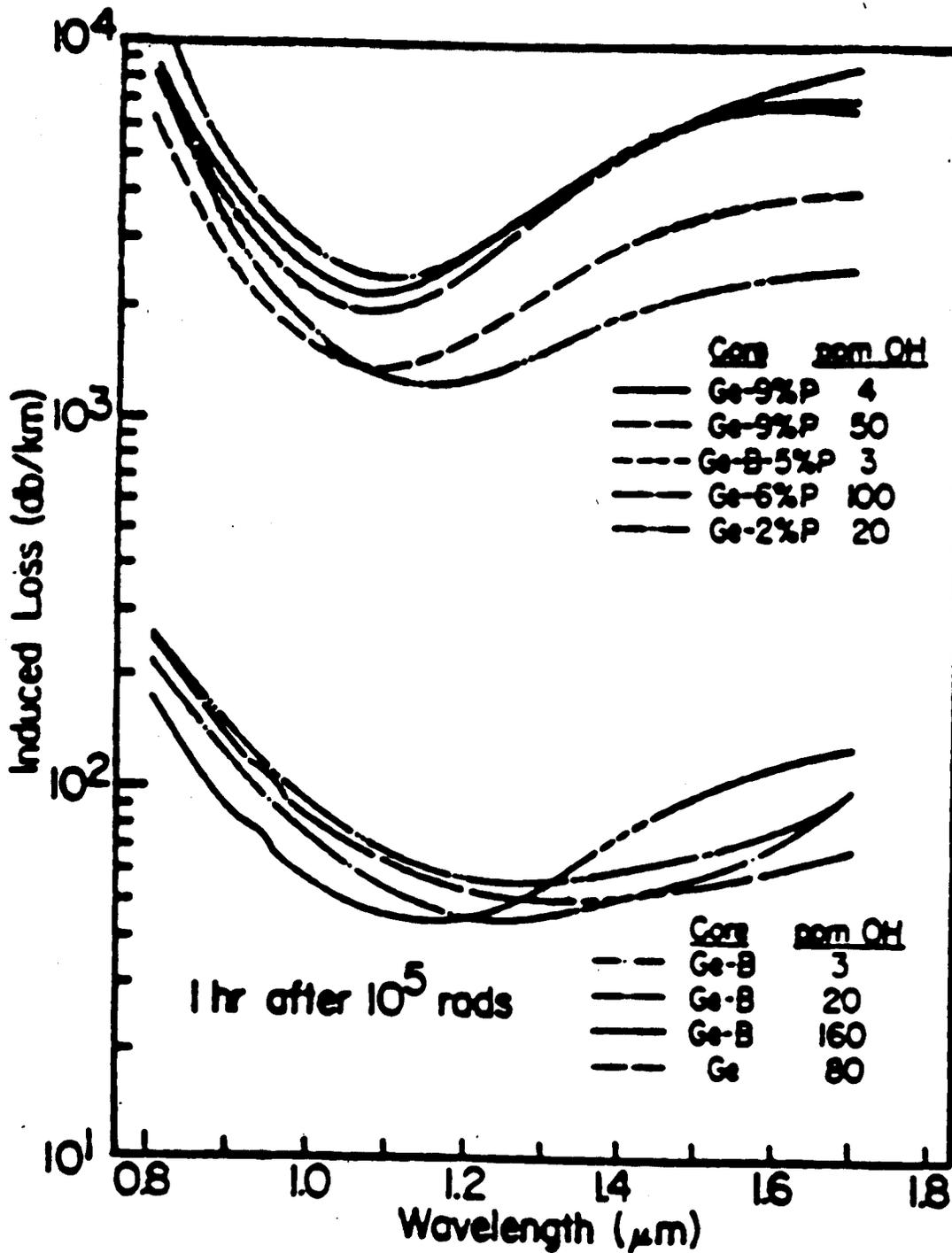
duced absorption of Ge-doped silica-core optical waveguide (0.67) was used to strip the cladding modes. Short dashed line shows the second OH overtone band at  $1.37 \mu\text{m}$  made determination of induced loss at  $1.37 \mu\text{m}$  although such changes could have been easily detected in fibers with induced loss at  $1.37 \mu\text{m}$  could be used with confidence in fibers with
