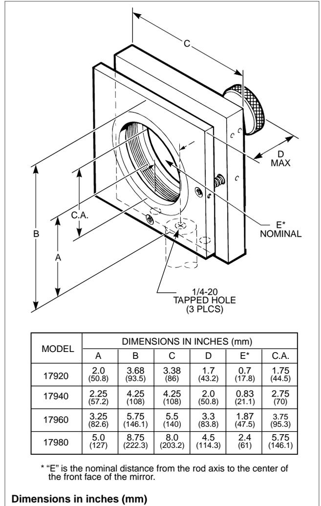
**Fig. 1 Dimensional diagram of Precision Adjustable Mirror Mounts.**
