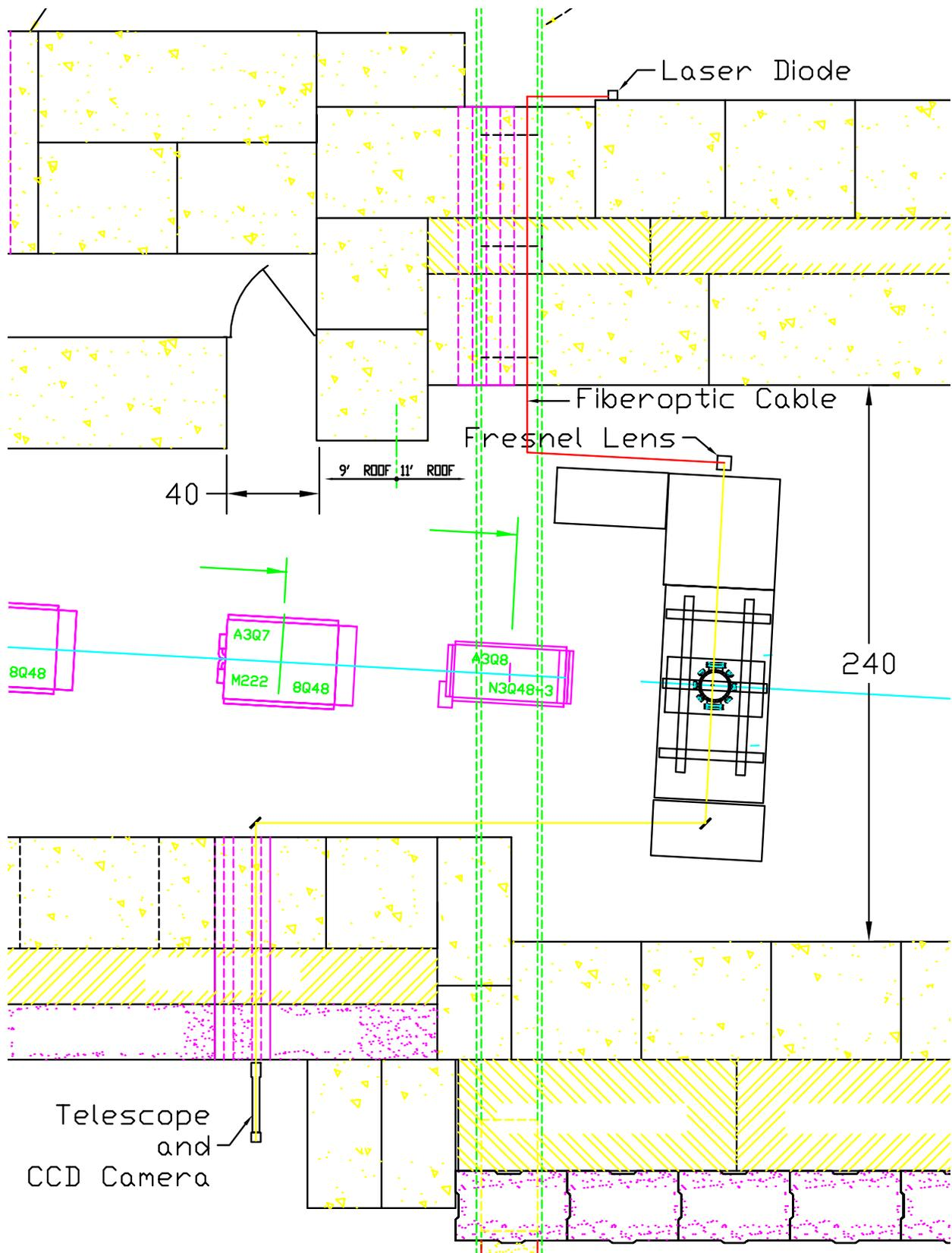
Figure 4: Layout of the optical transport between the laser diode and the high-speed camera in the A3 beamline for experiment E951.
