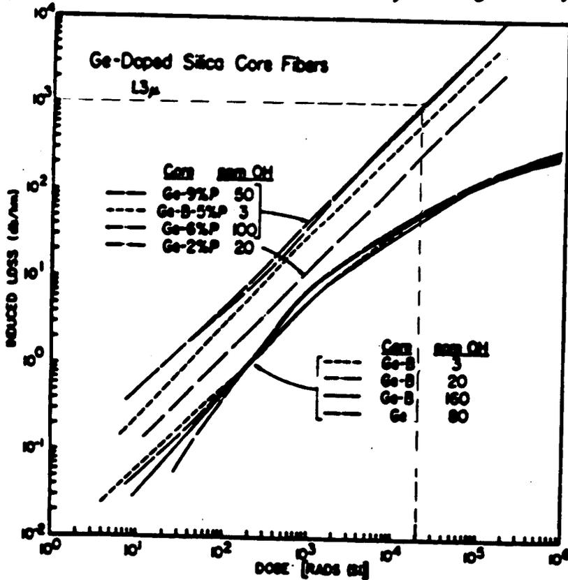
Fig. 3. Growth of radiation-induced attenuation at  $1.3 \mu\text{m}$  in Ge-doped silica-core fibers during steady-state irradiation. Note the decreased radiation response of these fibers at  $1.3 \mu\text{m}$  vis à vis  $0.82 \mu\text{m}$  (Fig. 2).
