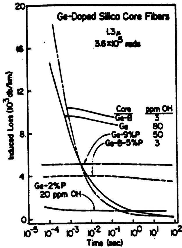
ig. 5. Time evolution of the radiation-induced attenuation of Ge-doped silica-core fibers at  $1.3\mu$  following a pulsed electron irradiation of 360,000 rad. Dose rate =  $1.2 \times 10^{14}$  rad/sec;  $T = 300$  K.
