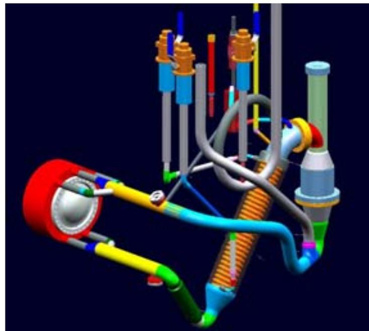
Forced-Flow with external cooling loop
