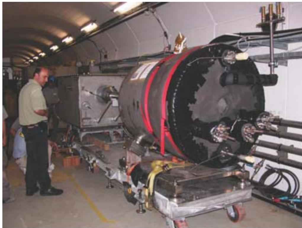
Magnet and Hg Jet system installed in TT2A tunnel at CERN
