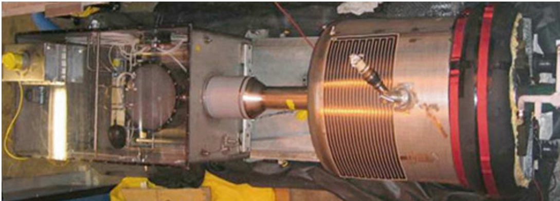
FIG. 6: Photographs of the entire MERIT experiment. a.) Sectional side view of mercury loop system integrated with 15 T solenoid magnet. b.) Fabricated mercury loop system assembled with 15 T solenoid magnet (Top view).
