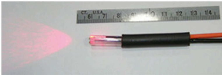
FIG. 2: Photograph of optical head assembly and its illumination of laser. a.) Front view of optical head assembly. b.) Side view of optical head assembly. c.) Illumination of fiber-optics head assembly.
