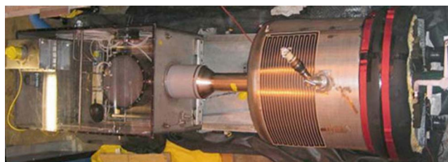
FIG. 6. (Color online) Photographs of the entire MERIT experiment. (a) Sectional side view of mercury loop system integrated with 15 T solenoid magnet. (b) Fabricated mercury loop system assembled with 15 T solenoid magnet (top view).
