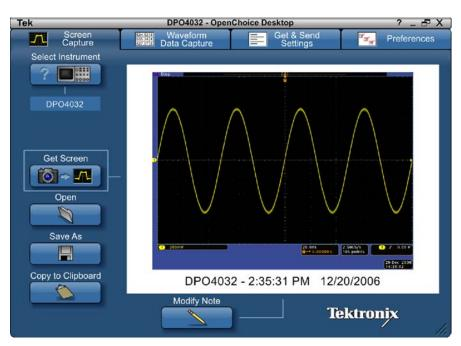
Figure 1: Tektronix OpenChoice Desktop
