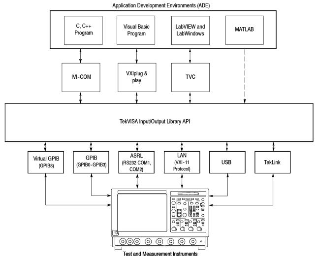
Figure 2: The relationship between programming interfaces
