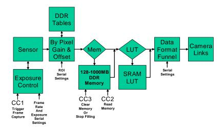
DDR Memory can be organized as a FIFO or as a circular buffer. CC3 is used to clear the memory (FIFO) or stop filling the memory (circular buffer). CC2 is used to read the top most images from memory (FIFO) or to read the oldest non-read image from memory (Circular buffer).
