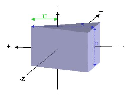
The wedge geometry can accept a second MTAG parameter in the SREGION construct. The first material refers to the interior of the wedge. The second material, if present, refers to the exterior of the wedge. If a second MTAG parameter is not present, vacuum is assumed.
