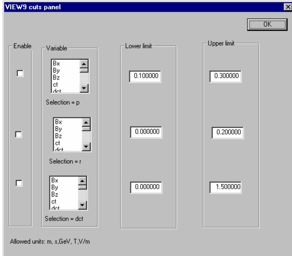
The user can enable up to three cuts on the plotted variables by checking the boxes on the left. The user can use one of the three default variables or choose another from the list of allowed variables. The accepted range must be entered in the lower and upper limit boxes.
