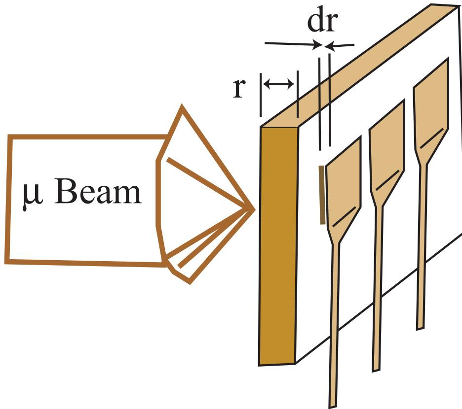
The  $r$  and  $dr$  measurements determine if the device is a Faraday cup or a SEM, the operation is similar.
