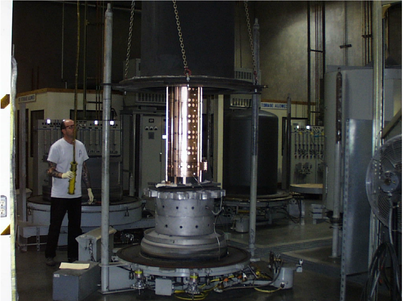
805 MHz open cell cavity after brazing
