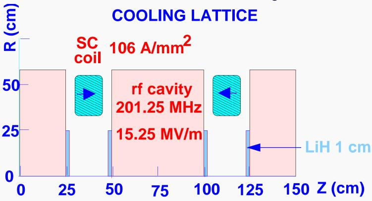
Beta function is constant  $\approx 80$  cm. Window are absorbers; they are 1 cm LiH with coating, 25 $\mu$ m of Be.
