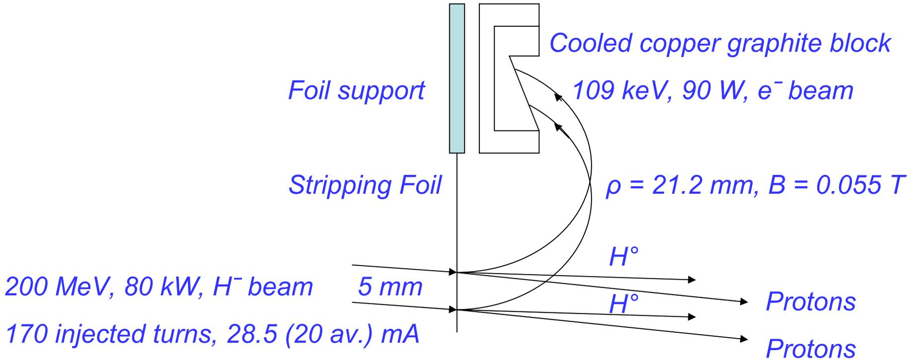
*Foil lattice parameters :  $\beta_v = 7.0 \text{ m}, \beta_h = 7.8 \text{ m}, D_h = 5.3 \text{ m}, D_h / \beta_h = 1.93 \text{ m}^{1/2}$*
