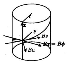
The field within a bent solenoid, far from its ends, is the same as that around a single vertical current I
