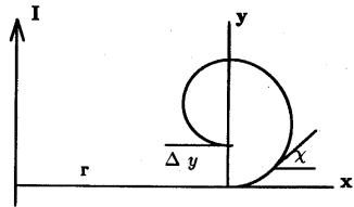
The bending radius  $\rho$  in the plane (x,y) including the current I is given by:
