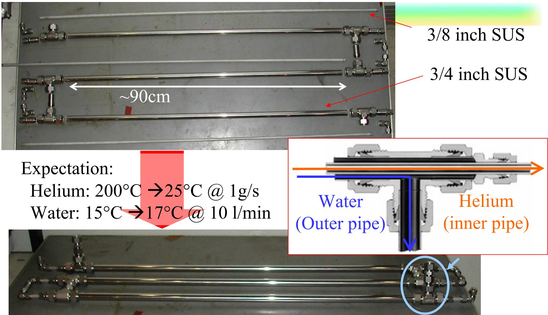
This heat exchanger has the purpose of the test of the water-jacket for the helium cooling pipe (1<sup>st</sup> heat exchanger) in the actual system.
