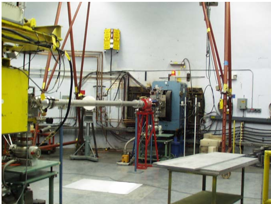
Target-2 with pipe in place for beam transport to Target-4
