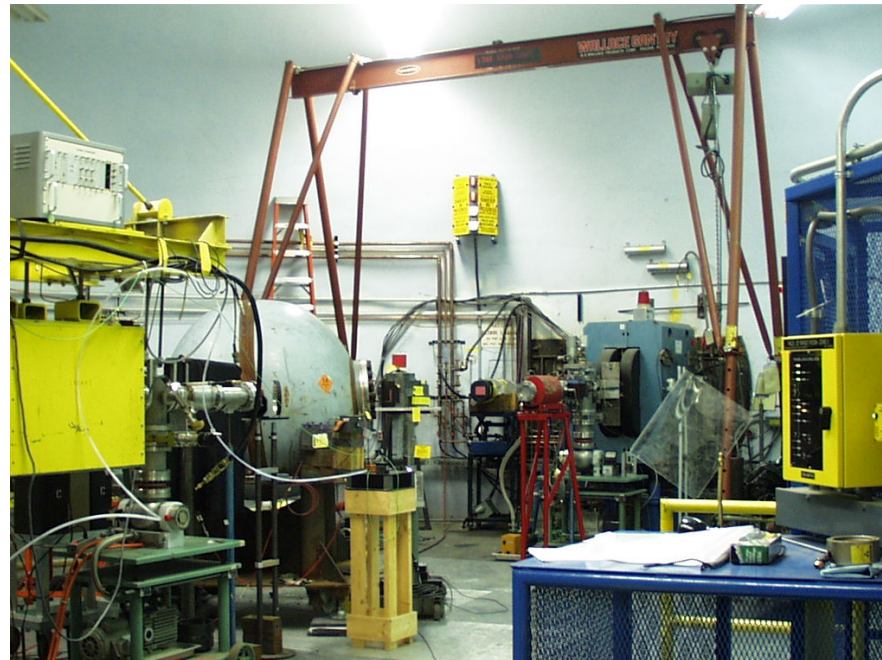
Target-2 with neutron production target and explosive containment vessel in place
