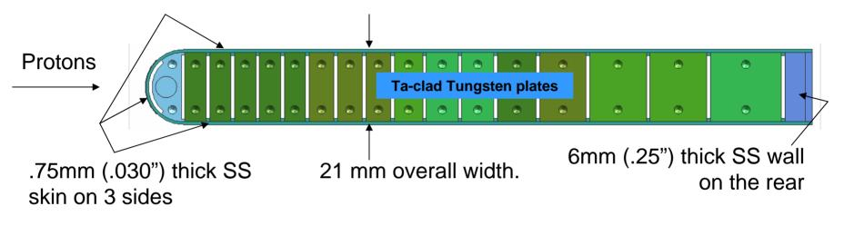
Sides are not bonded to the target plates. Target must be clamped between the fuel housing and material sample housing before applying internal coolant pressure.
