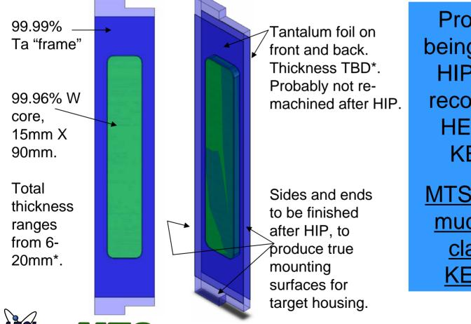
Prototypes now being made, using HIP parameters recommended by HEARO for the KENS target.
