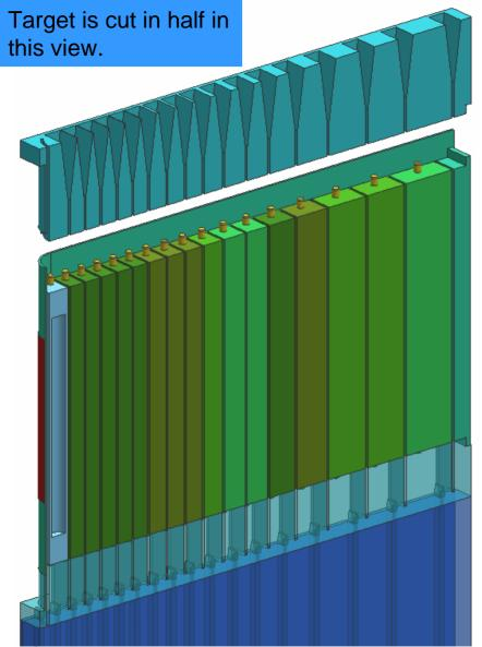
1mm wide passages carry D<sub>2</sub>O at 10m/s between W/Ta plates
