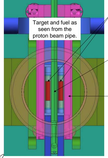
Two rectangular proton beam "spots" (15mmX60mm) are produced by painting <u>alternate macro-pulses</u> onto the two target halves.
