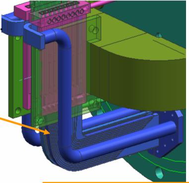
Elongated narrow channels shown. Orifices or labyrinth also being considered.
