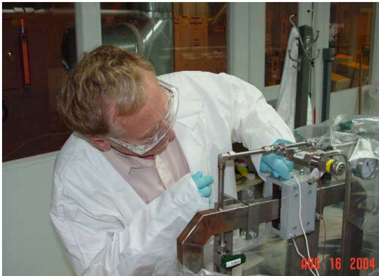
Dr. Imants Bucenieks from IPUL works on replacing the flow meter electrodes.
