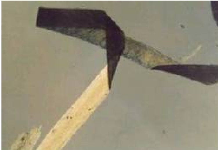
Fiber of carbon nanotubes (Heat transfer properties)
