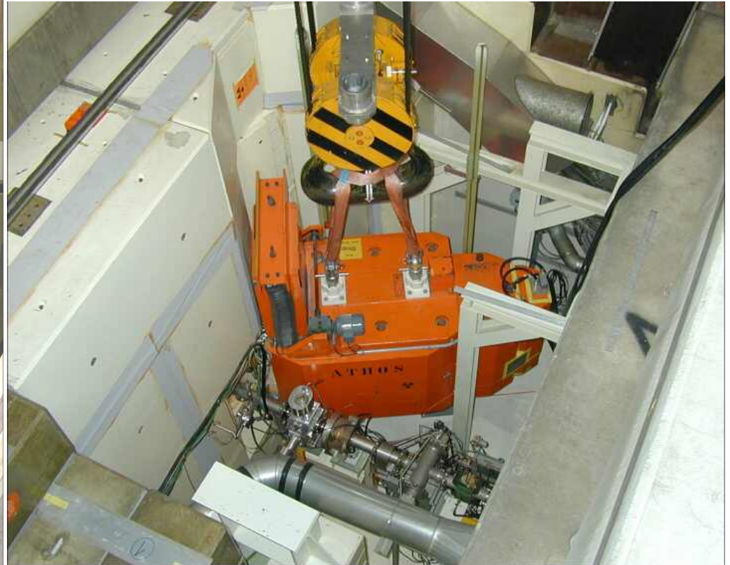
Operation of the remotely controlled shielded flask
