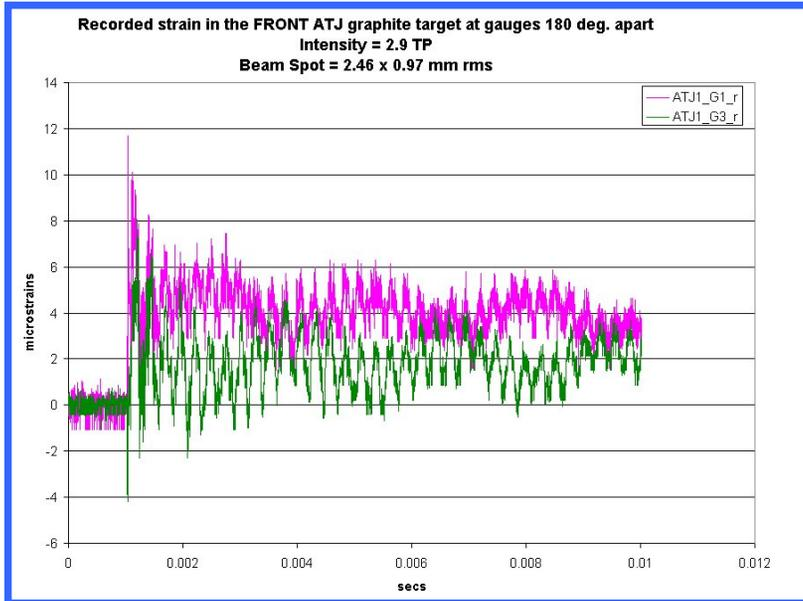
Record of strains in the middle of the graphite rod (left) shows a bending frequency between 380-390 Hz
