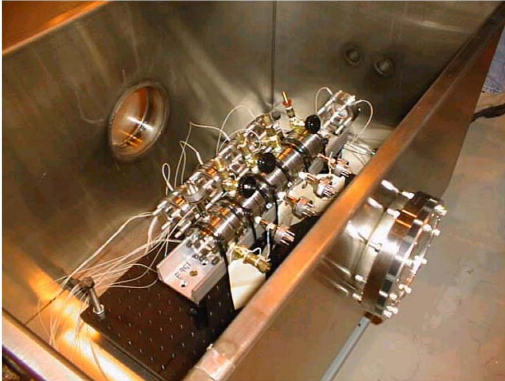
Fiberoptic Strain Gauge Arrangement in the 2" diam. Beam Window
