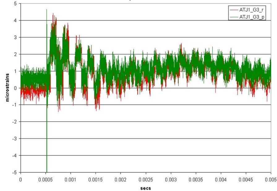
Recorded strain in the FRONT ATJ graphite target (mid-length)
