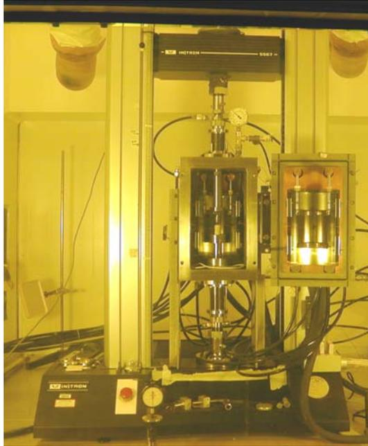
**Instron 5567 testing machine in recently installed Hot Cell:**
