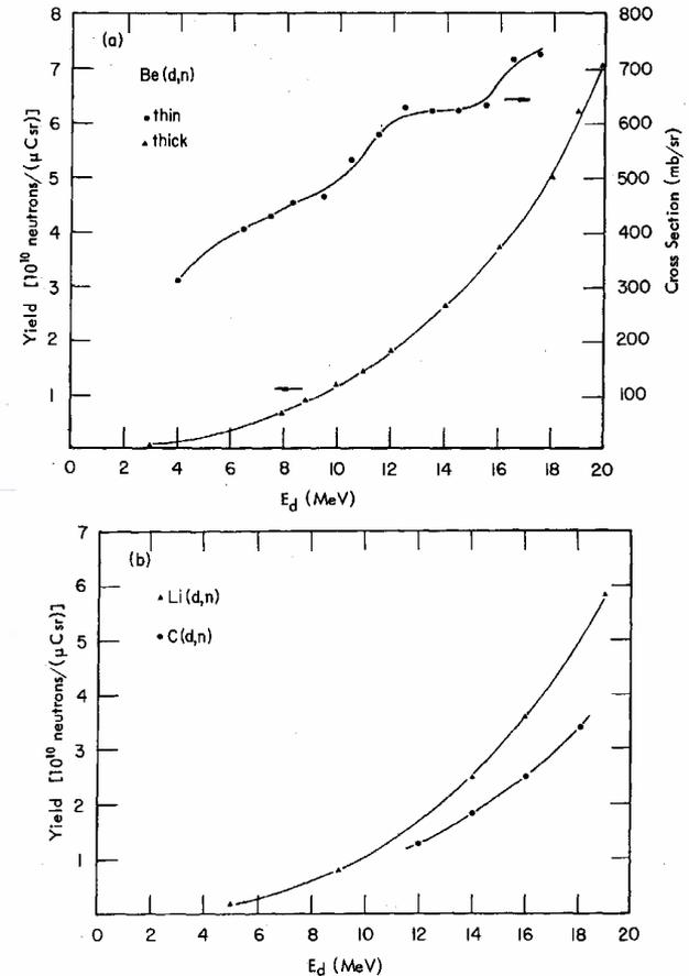
Fig. 5. Neutron production integrated over neutron energy for an emission angle of 3.5 deg as a function of deuteron energy: (a) yield for thick beryllium target and cross section for thin beryllium target and (b) yield for thick targets of lithium and carbon.
