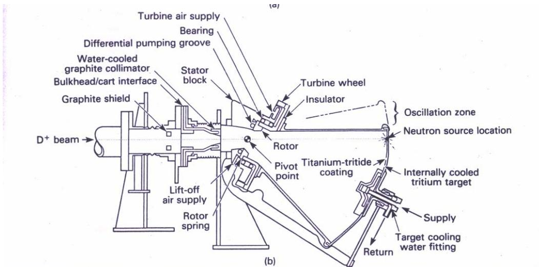
Fig. 3. (a) The externally cooled rotating target system used at RTNS-I, and (b) the internally cooled target assembly at RTNS-II.
